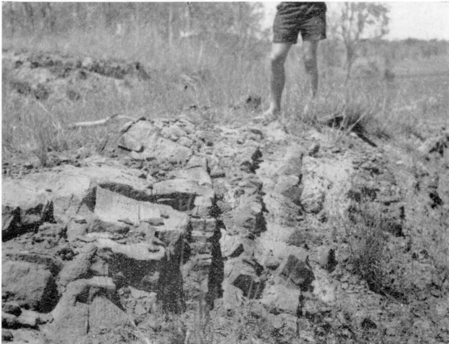
Plate 6a. Steeply dipping and probably faulted Marburg Sandstone in eastern flank of South Moreton Anticline (grid ref. 605513).
