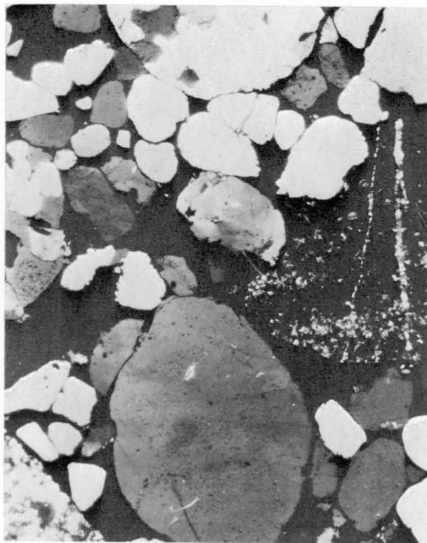
Plate 15, Figure 1. Granules of quartz, quartz sandstone, and microcrystalline quartz, and sand grains of quartz set in a matrix of hematite. Border Creek Formation, Mt Septimus (loc. 104-22A). Crossed nicols, x 20
