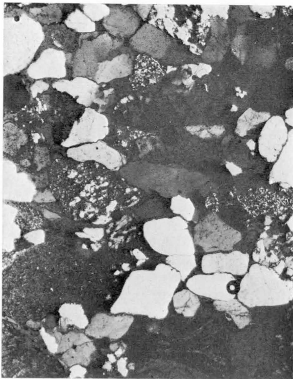
Plate 15, Figure 2. Grains of quartz, microcrystalline quartz, feldspar, and biotite, cemented by overgrowth quartz. Cecil Member, Kununurra (loc. 415-3). Crossed nicols, x 20
