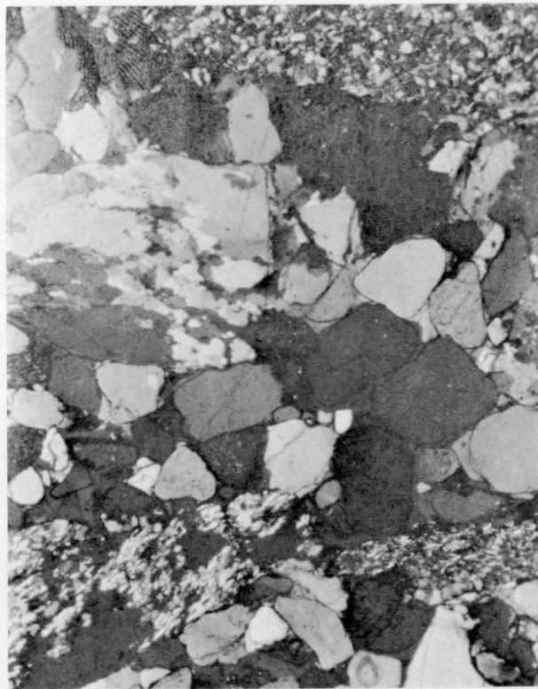
Plate 14, Figure 1. Rock fragments and quartz grains. Micaceous quartz siltstone (top and bottom) and vein quartz (middle left). Kellys Knob Member, Matheson Ridge (loc. 28-7). Crossed nicols, x 20
