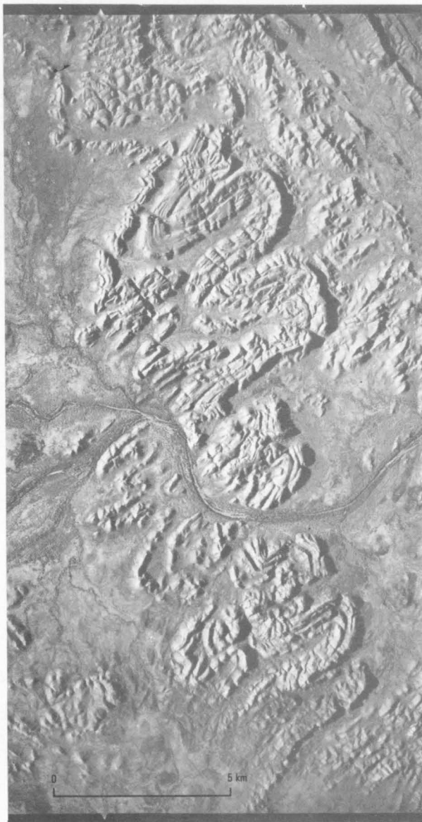
Fig. 57. Infrared airphoto of the area centred about 10 km east of Malbon, showing tight to isoclinal northeast-plunging large-scale folds in ridge-forming Mitakoodi Quartzite on the eastern side of the Malbon Block. These folds appear to die out to the west, in the underlying Marraba Volcanics and Argylla Formation, and do not persist above the overlying Overhang Jaspilite to the east. They appear to fold pre-existing cleavages associated with the Duck Creek Anticline, and hence probably postdate this structure. No folds of this style and orientation have been found elsewhere in the region.
