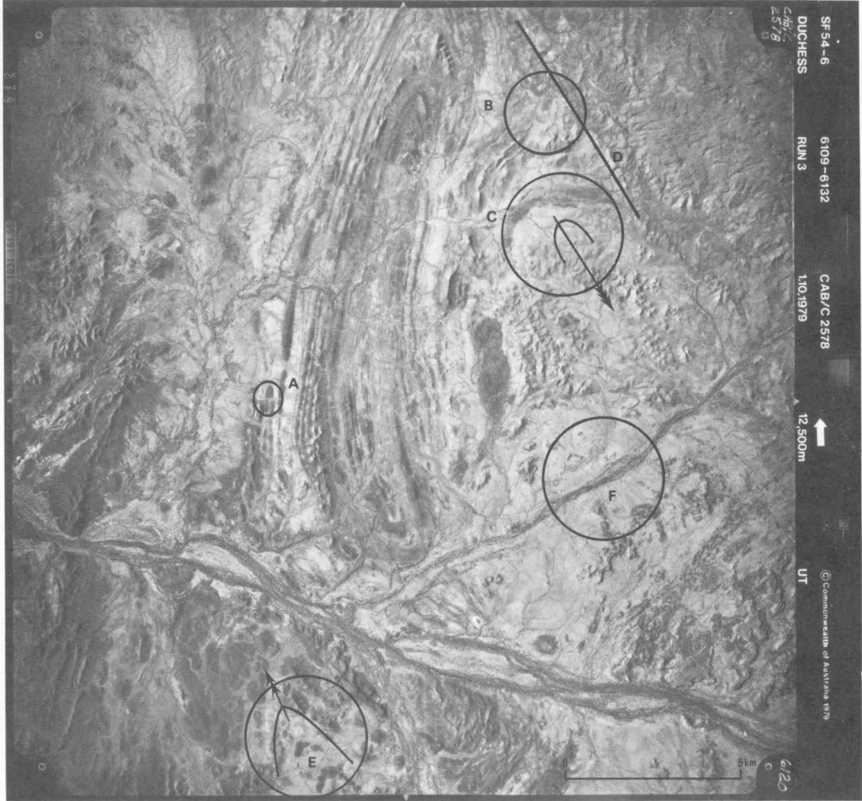
Fig. 46. Infrared airphoto of the area around Kuridala, showing a north-trending, probably second-generation, tight structural basin (synform), outlined by dark grey metadolerite sills, within the Kuridala Formation. The dominant layering in the Kuridala Formation in the synform is a first-generation schistosity which is generally parallel to bedding and the sills. A weak crenulation cleavage present in the hinge areas is parallel to the axial plane of the synform. Small-scale first-generation folding is inferred where bedding is at a high angle to the schistosity. Folded metadolerite to the west, at locality A, may define a first-generation fold. In the northeast, third-generation box folds at locality B and southeast-plunging open folds at locality C may be related to movement along the nearby Straight Eight Fault (labelled D). Northwest-plunging second-generation folds are evident in the Kuridala Formation at E, in the south. A post-tectonic granite body, mapped as Squirrel Hills Granite, forms subdued terrain in the east, near locality F.
