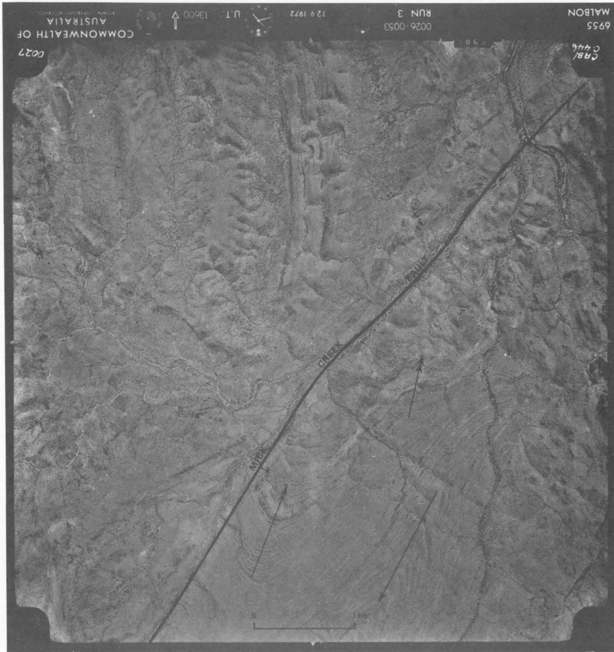
Fig. 59. Airphoto of an area centred 22 km north of Kuridala, showing well-bedded calc-silicate rocks of the Doherty Formation in the south, the northeast-trending Mick Creek Fault, and north-trending ridges of westerly dipping Roxmere Quartzite? in the north and northwest. The bedded calc-silicate rocks show two generations of folding—a south-southwest-plunging first-generation fold (single arrowhead) and north-northeast plunging second-generation folds (double arrowheads). The hilly terrain to the east and northeast is formed of calc-silicate breccia.
