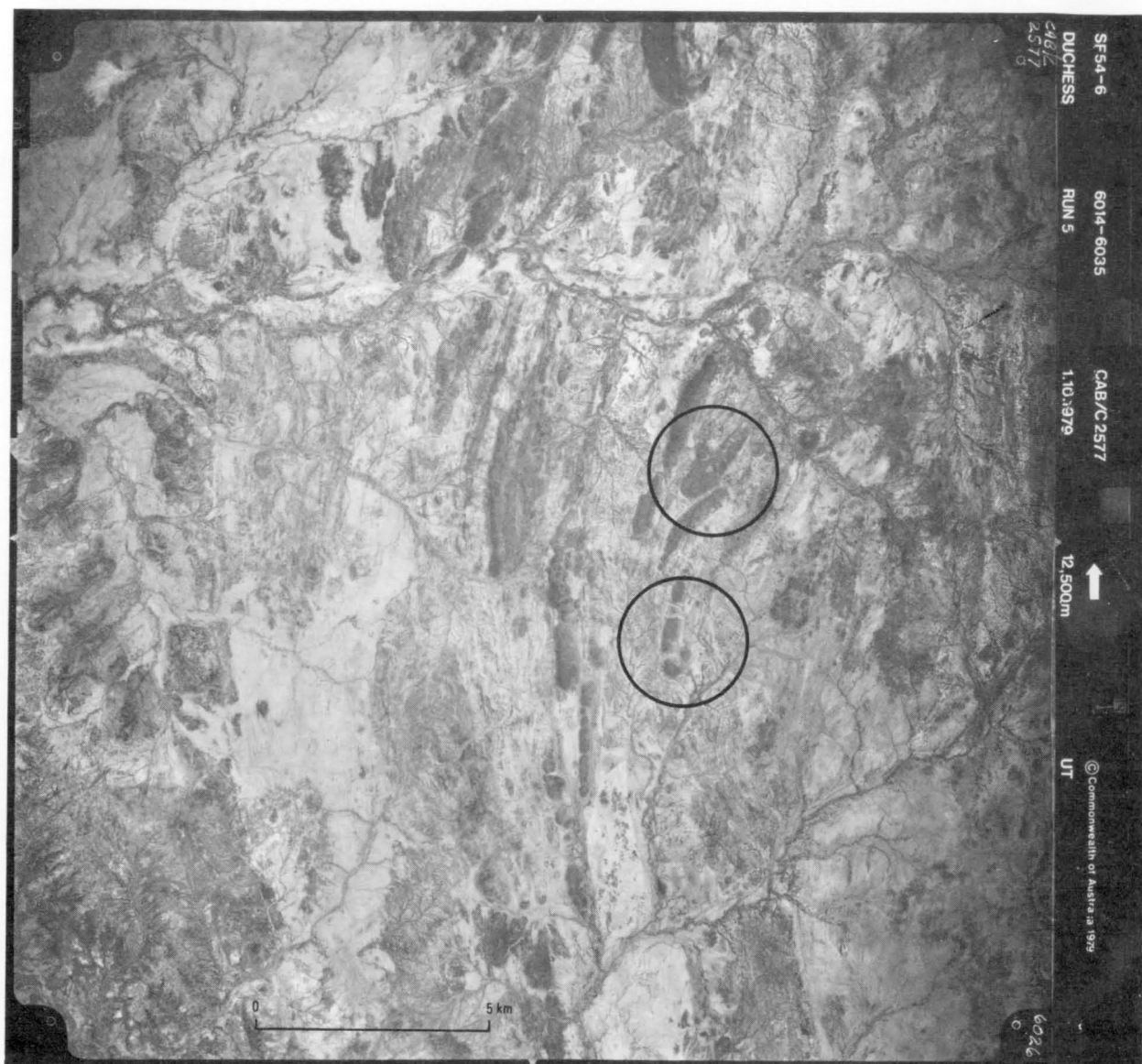
Fig. 44. Infrared airphoto of the area centred about 20 km west-southwest of Selwyn, showing metadolerite sills (dark grey) within the Mitakoodi Quartzite, Answer Slate, and Staveley Formation. The sills in the circled areas outline tight to isoclinal first-generation folds with axial planes parallel to the prevailing first-generation cleavage in the adjacent Answer Slate.
