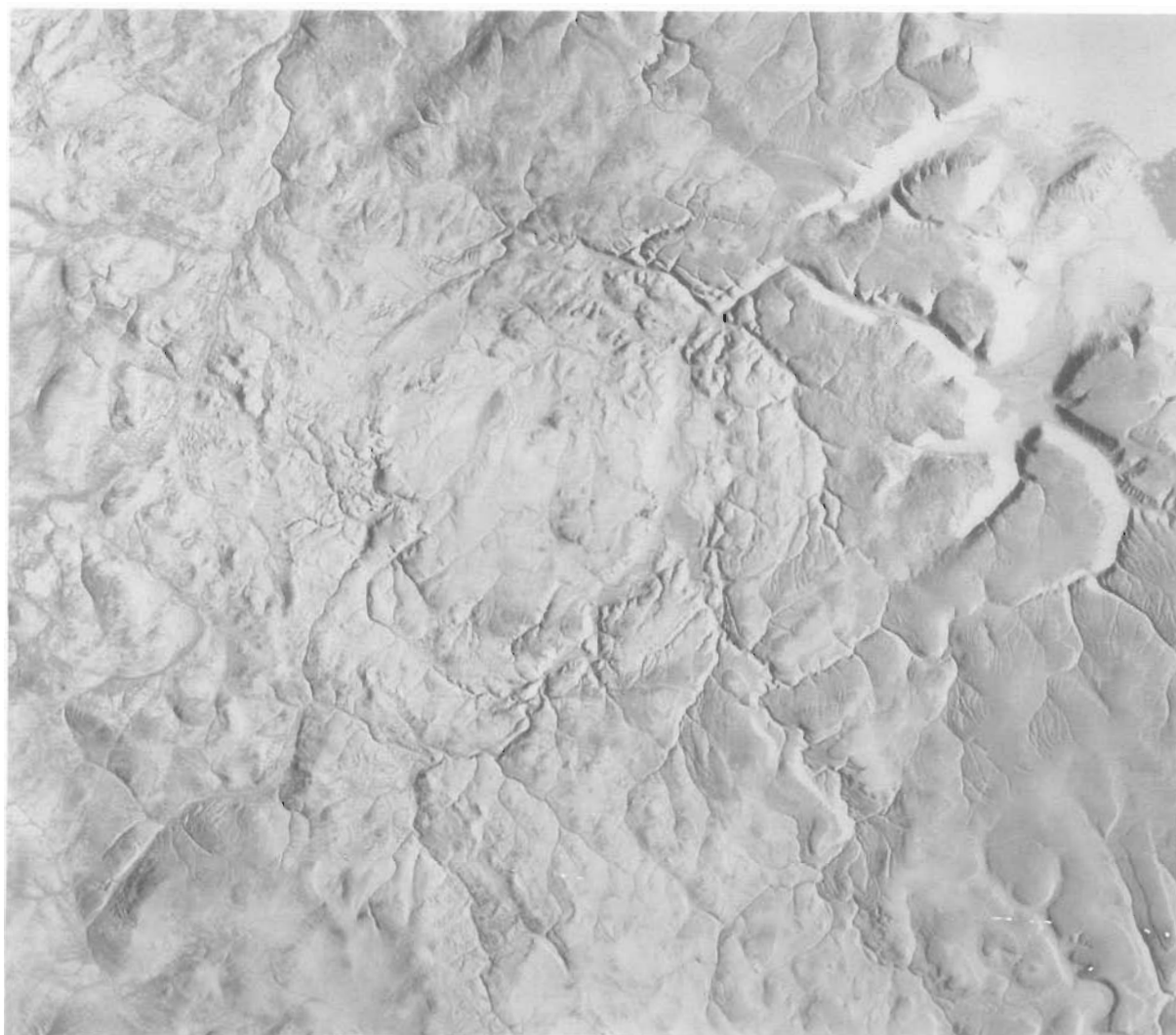
Figure 5. Airborne X-band radar image of the 24-km-diameter complex impact structure at Houghton (Canada; Table 1). Although only slightly eroded, it has no evidence of a topographic central peak (cf. Fig. 4).
