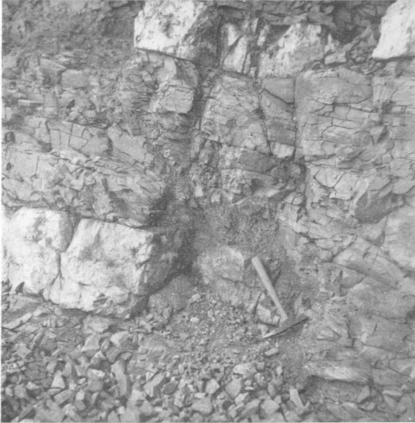
Fig. 5—Quartz vein displaced by reverse faulting; throw three feet. Hammer lies along fault plane.
