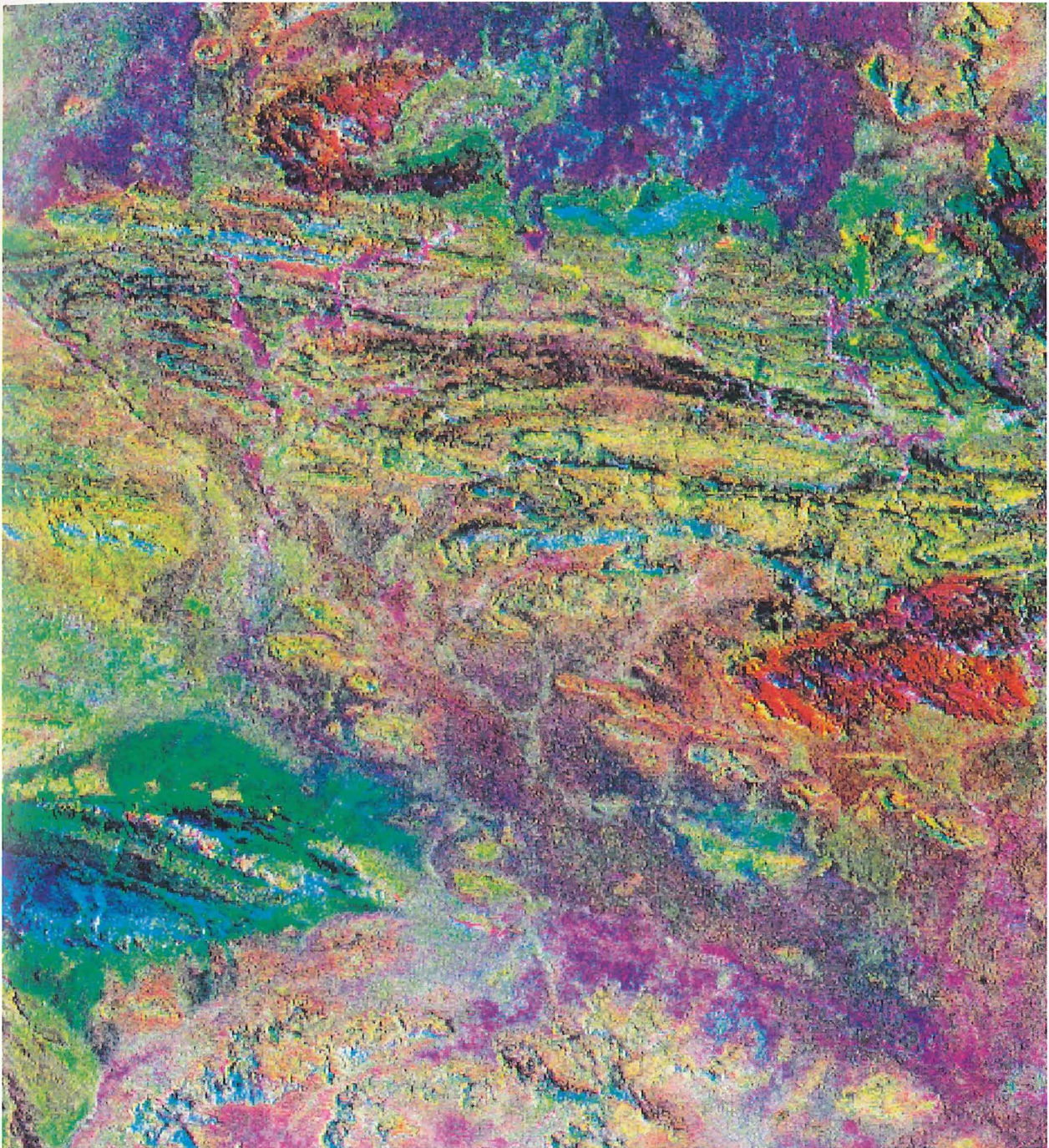
Figure 53. Landsat-5 TM pc2(4/3;5/7):5/4:4/3 RGB image of the Gosse Pile–Teizi bore area. The image includes part of the Gosse Pile pyroxenite intrusion (bottom left). Pyroxenite units (Px) are dominated by iron oxide-rich weathering crusts, and the different shades of green reflect the importance of this component; clinopyroxene–plagioclase-rich rocks have higher clay contents in their weathering crust and thus include a red component, giving a yellow signature. The deeply weathered serpentinised peridotite strike depression is characterised by calcrete–magnesite crusts showing in red and white. Shed iron oxide-rich alluvial material shows in deep apple green (Mc). Shaded southern slopes (Ss) display green vegetation superposed on pyroxenite bedrock, resulting in deep azure blue. The Teizi anorthosite suite includes several massive bodies (An) and numerous thin recrystallised tongues intercalated with felsic granulite (Fg). Anorthosite shows in red, representing clay–carbonate-dominated weathering, and felsic granulite in green and yellow tones, representing iron oxide–clay mixtures. Landsat discrimination of thin recrystallised anorthosite units is much more efficient than time-consuming field work. The sequence is cut by west to northwest-striking mafic dykes (Md). Alluvium derived from felsic granulite is typically clay-rich (Fc), showing in red or purple where supporting green vegetation.
