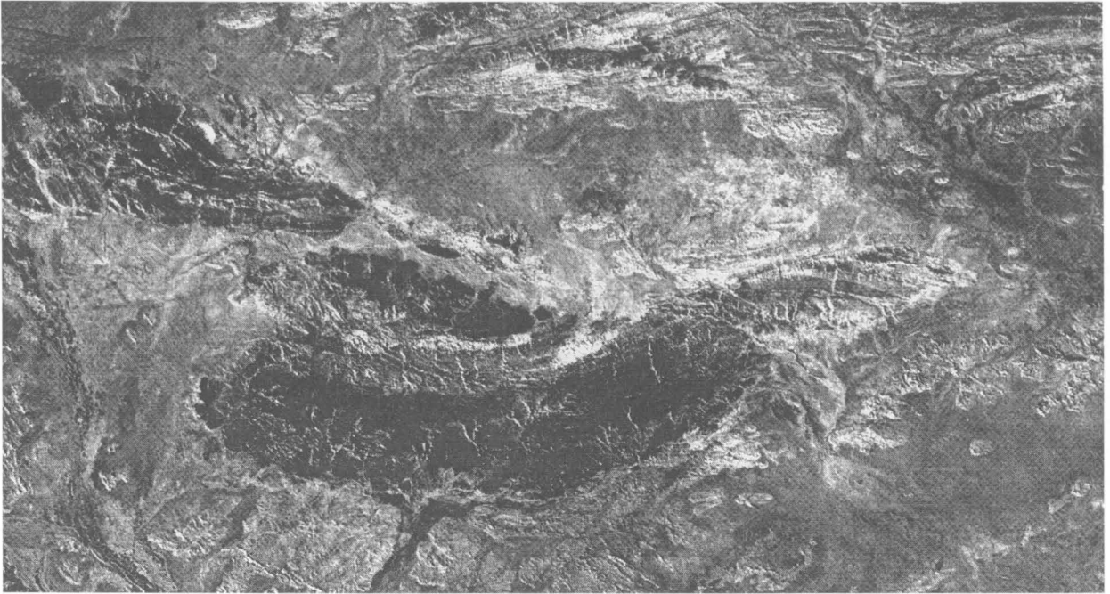
Figure 56. Landsat-5 TM 5/4 band ratio image of the Mount Davies–Kalka area. Light areas represent iron oxide-rich laterite and iron oxide-rich weathering surfaces of pyroxenite and felsic granulite. Compare with Figure 50.
