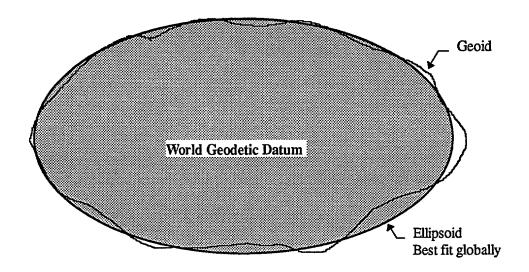
Calculated positions from the GPS are in the World Geodetic System 1984 (WGS84). The WGS84 datum is a global geocentric reference datum that has as its origin the Earth's centre of mass.
