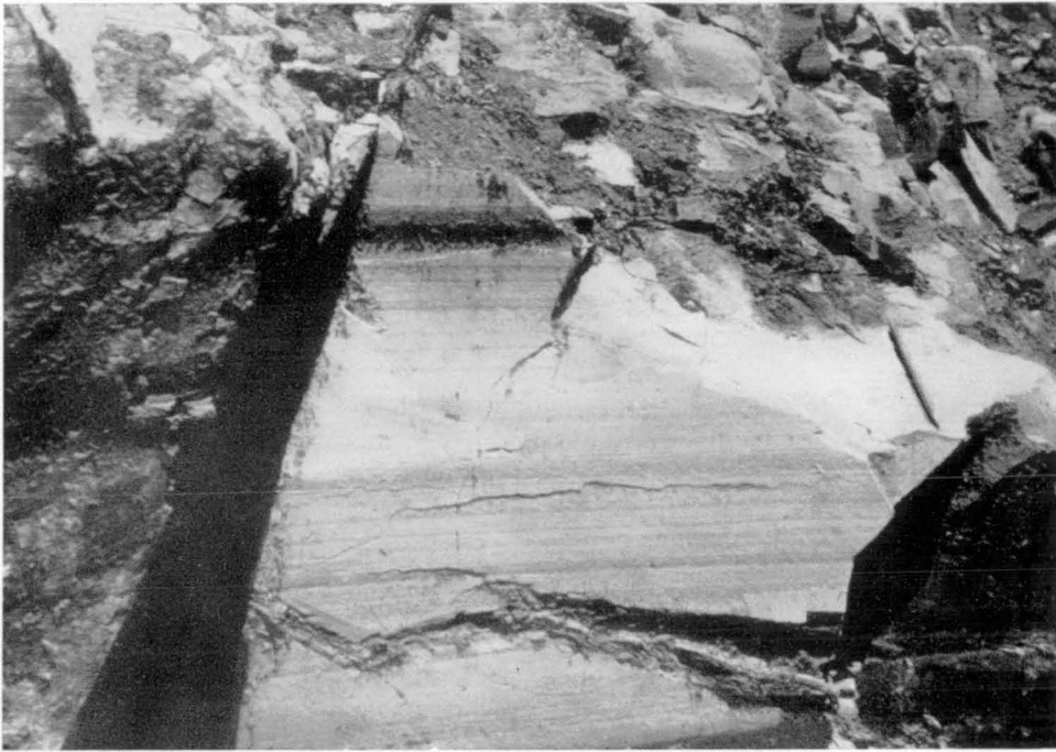
Fig. 18. Bedding in Silurian soft calcareous mudstone (City Hill Shale) in trench at Olympic Pool, Constitution Ave. The pencil is on a bedding plane (dip 32^{\circ} E.).
