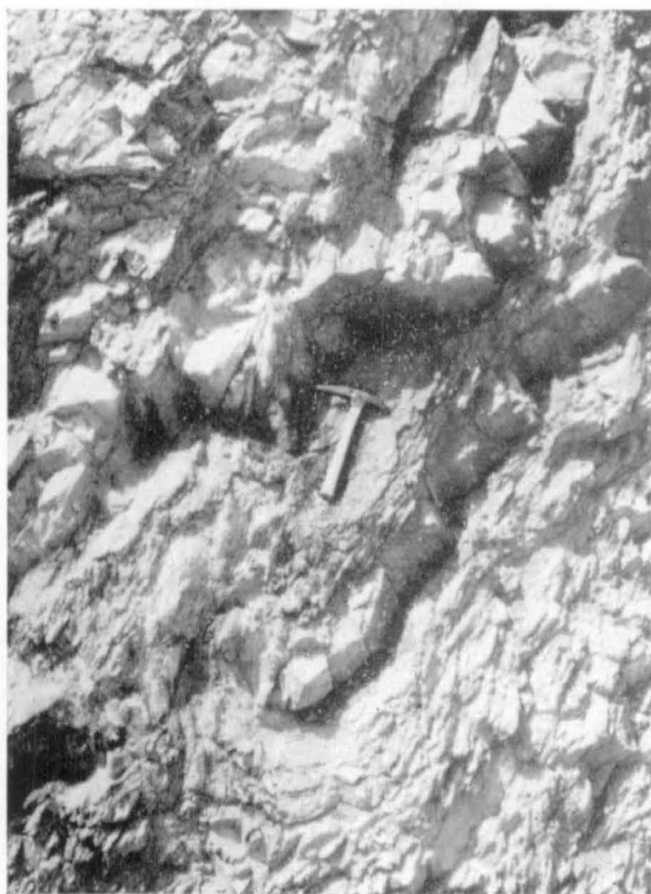
Fig. 12. Foundation of Medical School, Acton. Contorted interbedded shale and sandstone of the Pittman Formation. The structure consists of disrupted close folds steeply plunging towards the reader. See also Fig. 13.
