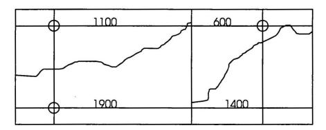
When you arrive at the time at which the depth scale changes, press "9" on the cursor keypad and you will be prompted to enter the new *top depth* and *bottom depth* at the keyboard. Continue digitisation after changing the depth scale.
