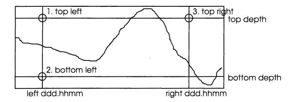
As implied in the diagram, you don't have to limit your digitisation to the area within the rectangle defined by points 1, 2 and 3. You can digitise beyond the limits of left ddd.hhmm and right ddd.hhmm, as long as the paper speed remains constant throughout. If the paper speed changes, you will have to start a new section and define the reference points again.
