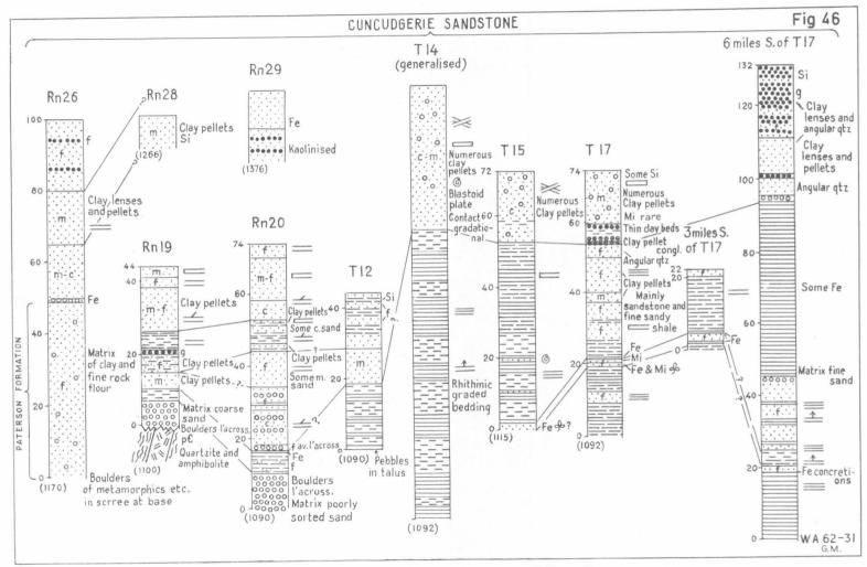
Fig. 46.—Sections of Cuncudgerie Sandstone, Runton and Tabletop Sheet areas.
