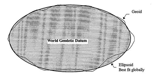
Calculated positions from the GPS are in the World Geodetic System 1984 (WGS84). The WGS84 datum is a global geocentric reference datum that has as its origin the Earth's centre of mass.
