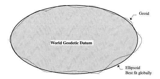
Calculated positions from the GPS are in the World Geodetic System 1984 (WGS84). The WGS84 datum is a global geocentric reference datum that has as its origin at the Earth's centre of mass.
