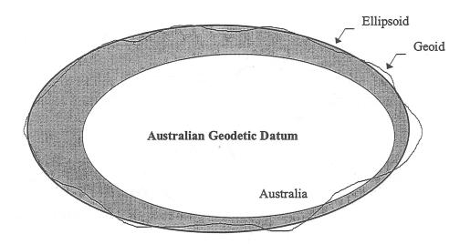
Calculated positions from the GPS are in the World Geodetic System 1984 (WGS84). During processing these positions are converted to the local reference datum, AGD84 or Australian Geodetic Datum 1984.
