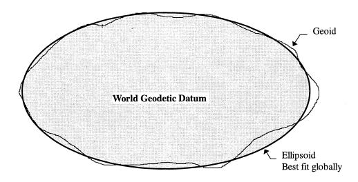
Calculated positions from the GPS are in the World Geodetic System 1984 (WGS84). The WGS84 datum is a global geocentric reference datum that has as its origin at the Earth's centre of mass.
