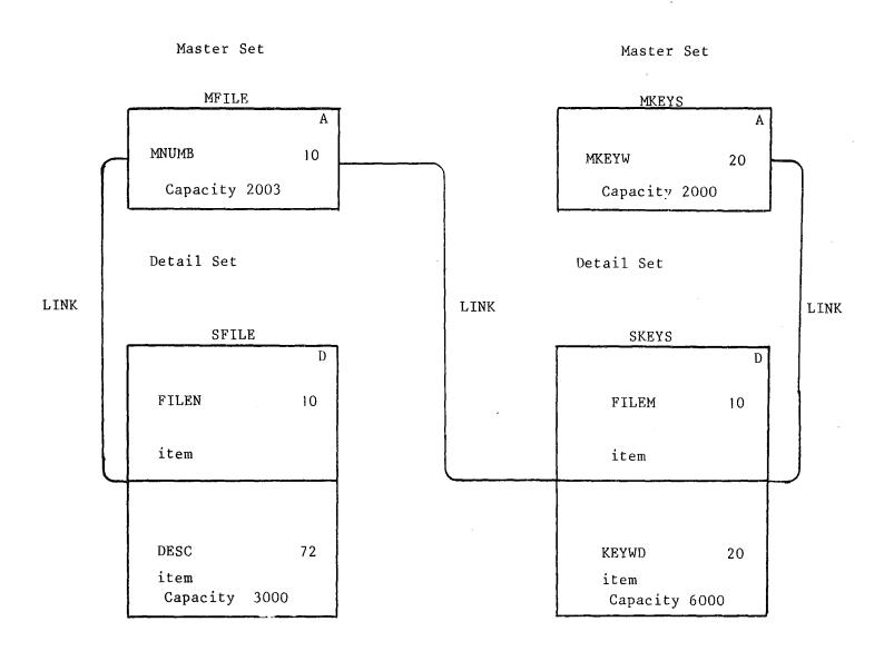
Fig. 1: Flow diagram for the REFIL data-base schema
