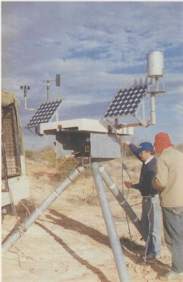
Pl. 6. Groundwater levels and climatic parameters are measured electronically and data transmitted by satellite, in remote parts of central Australia.
