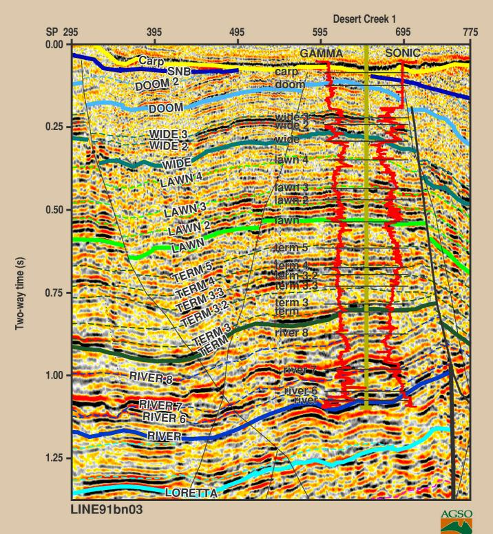
Figure 5.1.3 Desert Creek 1 well tied to seismic line 91bn-03
