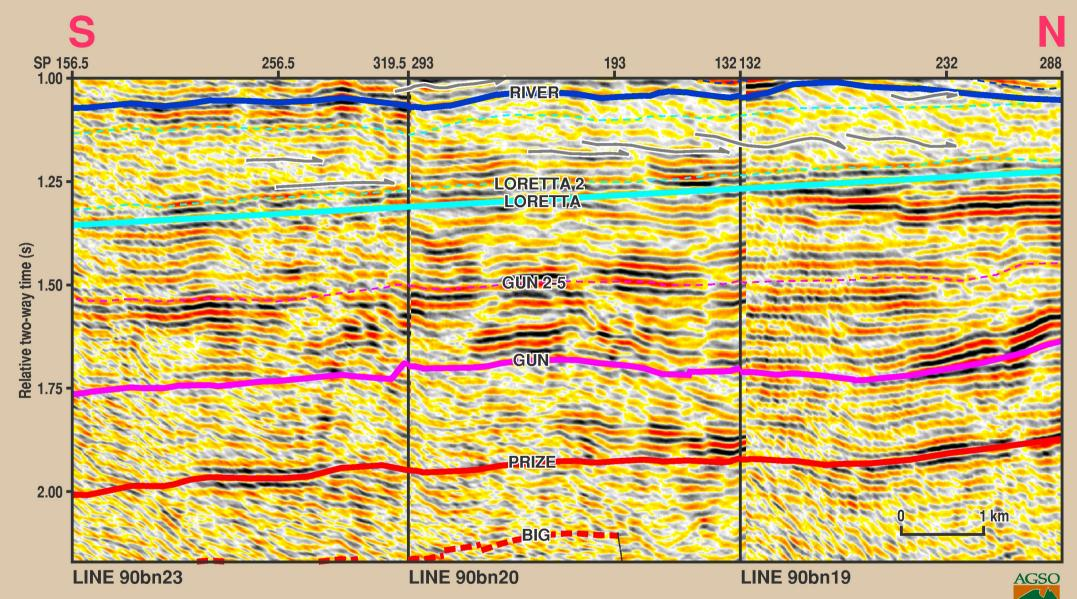
Figure 2.5.3 Seismic sequence stratigraphy of the Loretta Supersequence showing progradation of deformed evaporites over deeper marine carbonates, Lines 90bn-23, 20 and 19 (flattened on River). This figure is part of the Argyle Creek composite (Fig. 2.1.2)
