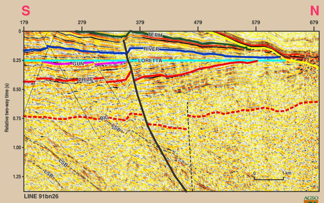
Figure 2.2.4 Seismic sequence stratigraphy of Big, Prize, Gun and Loretta Supersequences truncating Leichhardt Superbasin reflections, Line 91bn-26 (flattened on Loretta)
