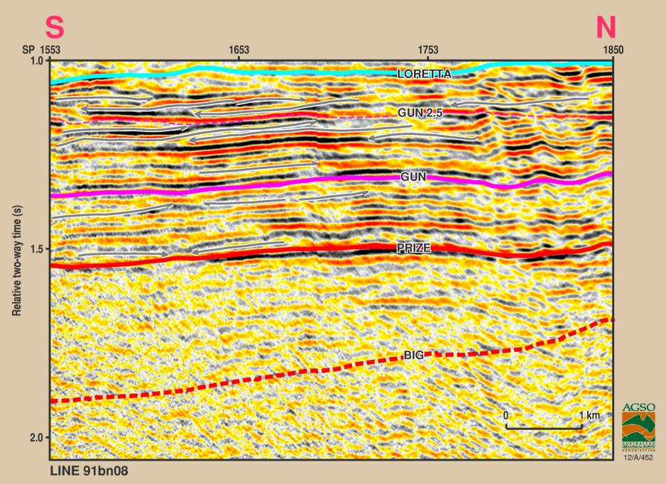
Figure 2.3.1 Seismic sequence stratigraphy of the Prize and Gun Supersequences, Line 91bn-08 (unflattened)
