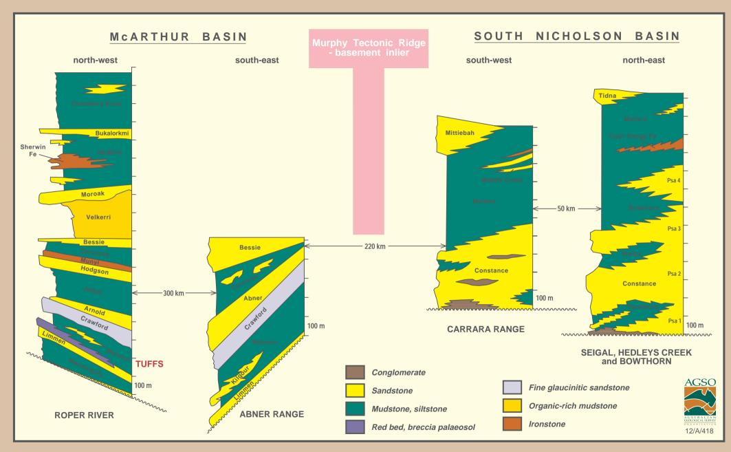
Fig 1.7.6 Representative lithostratigraphic sections through the Roper Group in the southern part of the McArthur Basin and the northern part of the Lawn Hill Platform
