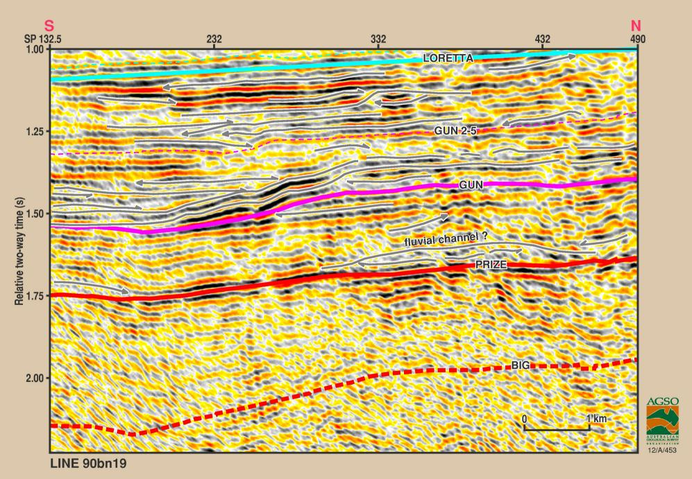
Figure 2.3.3 Seismic sequence stratigraphy of Prize and Gun Supersequences, Line 90bn-19 (unflattened). This section is part of the Argyle composite line (Fig. 2.1.2)
