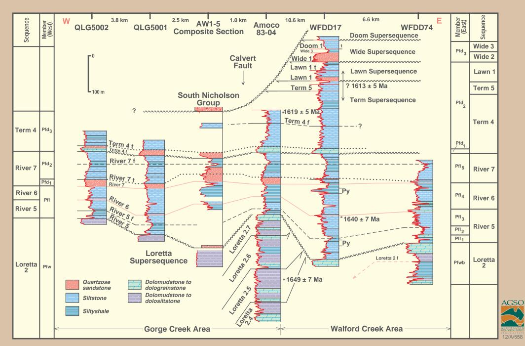
Figure 1.6.4 Cross-section of the Loretta through Doom Supersequences along the Murphy Inlier
