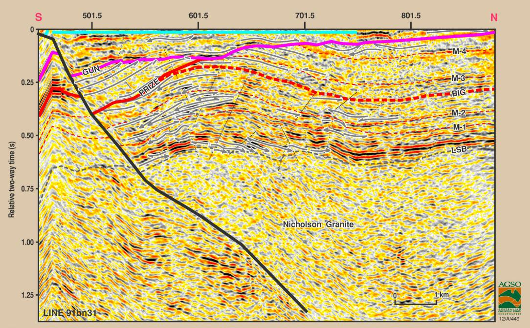
Figure 2.2.2 Seismic sequence stratigraphy of Big, Prize and Gun Supersequences over the Peters Creek magmatic dome, line 91bn-31 (flattened on Loretta). LSB = Leichhardt Superbasin. M1-M5 relate to magmatic members of the Peters Creek Volcanics. This section comprises the northern end of the Desert Creek composite Line (fig 2.1.3)
