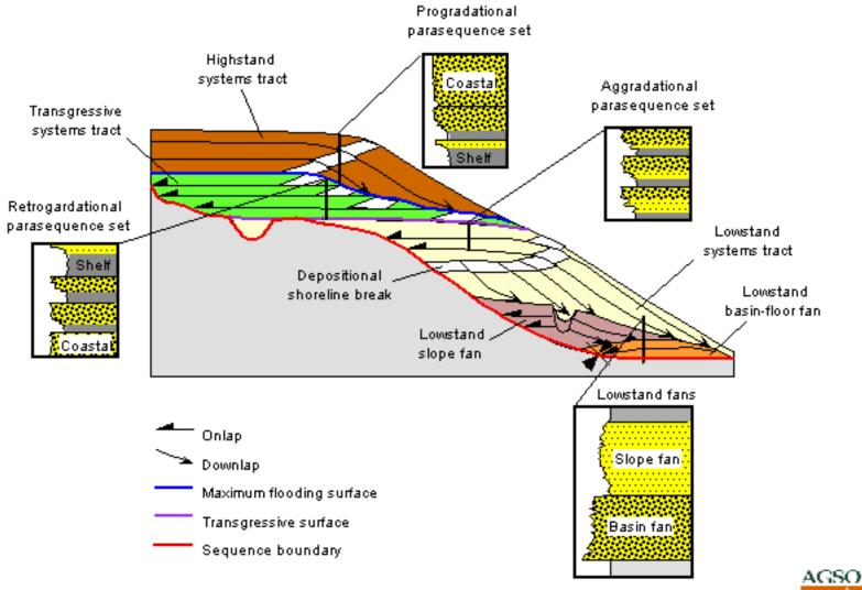
Figure A1 Geometry of parasequences defined by terminations that mark surfaces separating systems tracts
