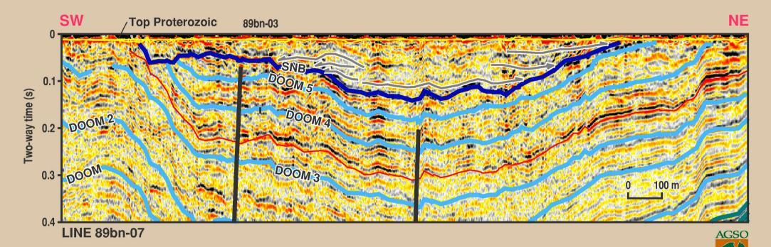
Figure 1.7.4 Seismic example of locally conformable relationship between South Nicholson Group (SNB) and Isa Superbasin. This relationship suggests deposition of the SNB commenced before deformation caused topography was fully peneplaned
