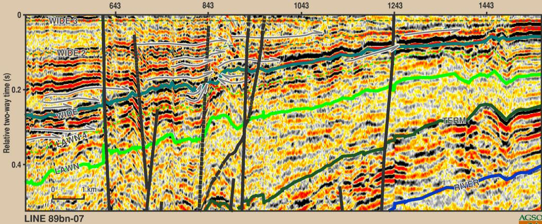
Figure 2.9.2 Seismic sequence stratigraphy of the Wide Supersequence showing onlapping geometry, Line 89bn-07 (flattened on Wide 3)
