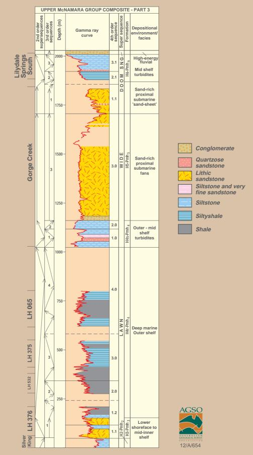
Figure 1.4.4 Composite gamma-ray and lithofacies logs for the Lawn, Wide and Doom Supersequences
