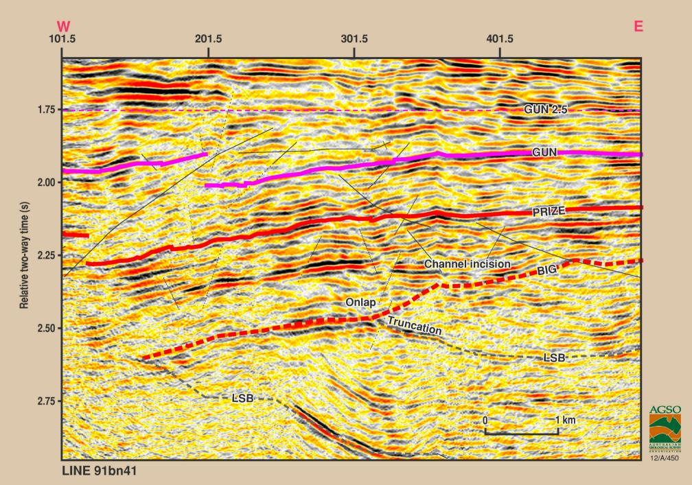
Figure 2.2.3 Onlap and insision of the Big Supersequence, showing angular unconformity with reflection interpreted as the Eastern Creek Volcanics (ECV) of the Leichhardt Superbasin, Line 91bn-41 (unflattened)
