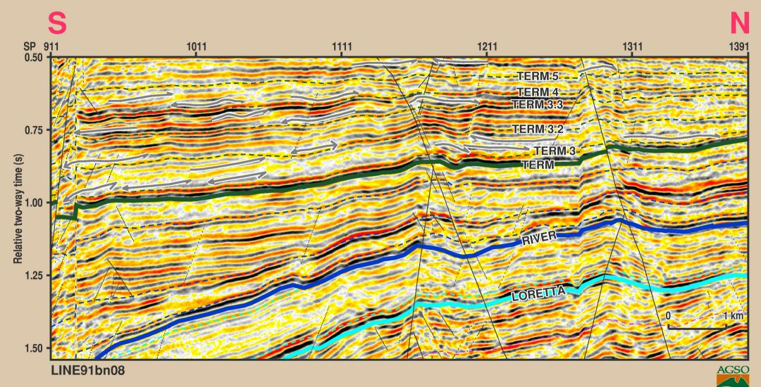
Figure 2.7.4 Seismic sequence stratigraphy of the Term Supersequence showing fan and channel levee geometry, Line 91bn-08 (flattened on Lawn)
