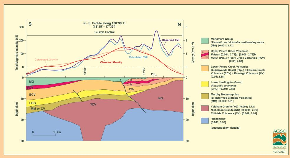
Figure 3.2.3 Geological model from the western side of the Comalco seismic grid compared to observed geophysical data
