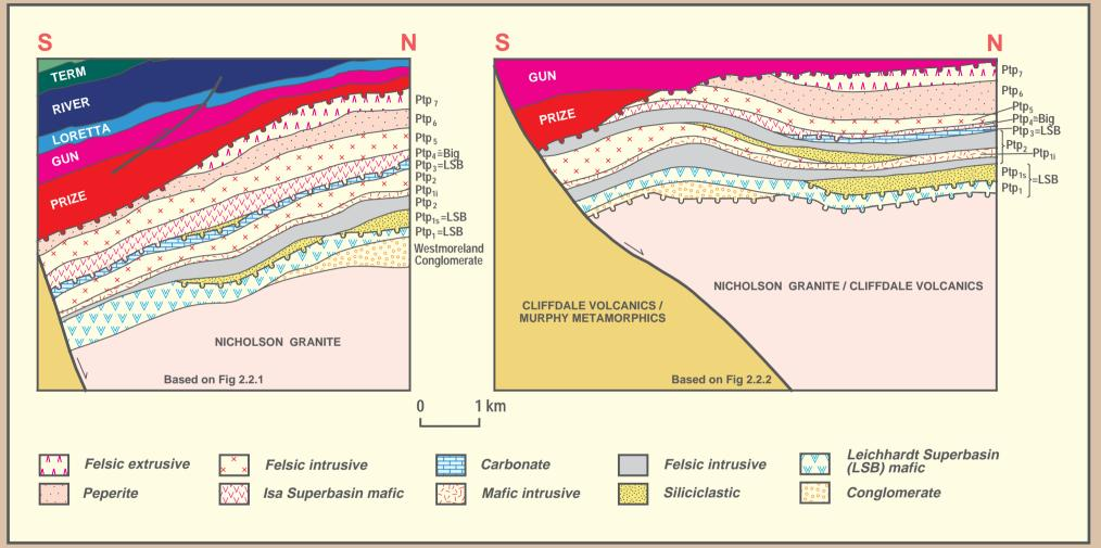
Figure 1.5.5 Geological interpretations of the seismic data (Figs. 2.2.1 and 2.2.2) that image the Murphy Inlier.
