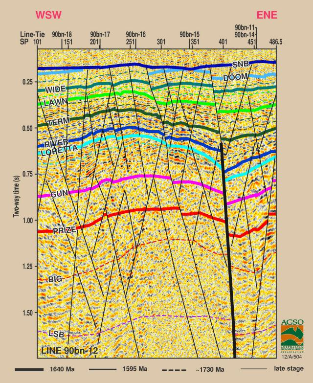
Figure 3.3.10 Late stage conjugate fractures
