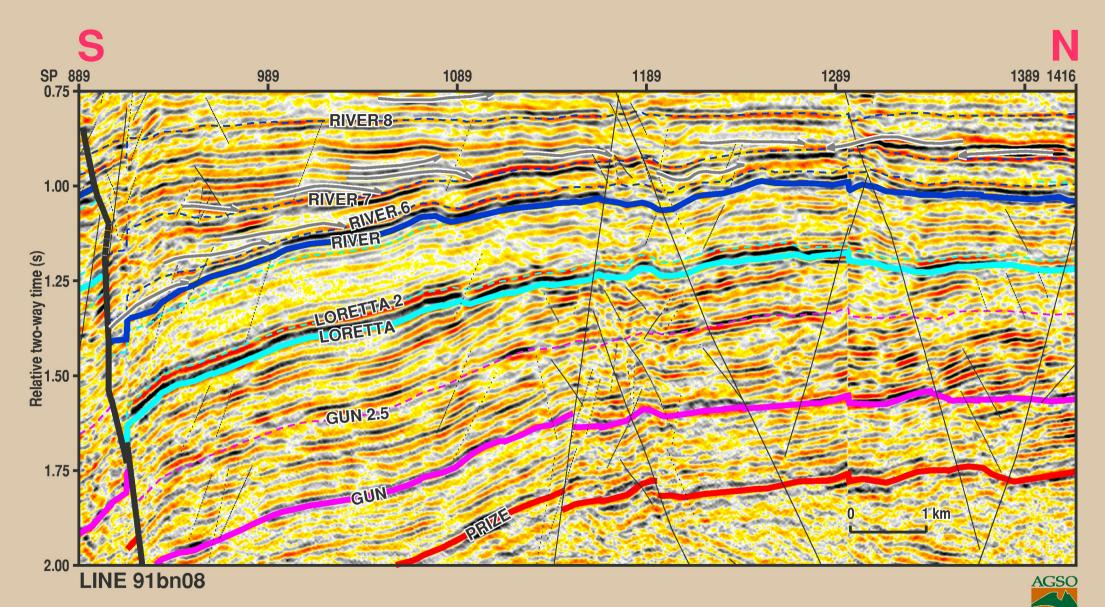
Figure 2.6.3 Seismic sequence stratigraphy of the River Supersequence showing tectonic wedges in the hanging wall block, Line 91bn-08 (flattened on term)
