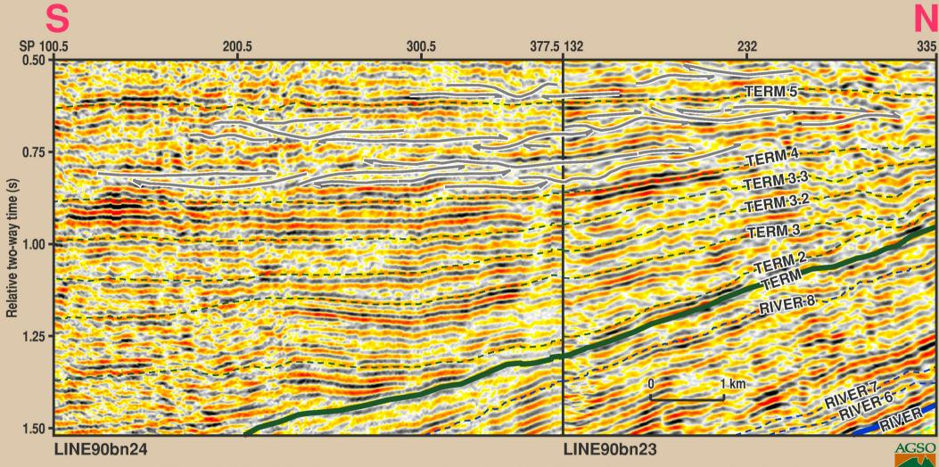
Figure 2.7.3 Seismic sequence stratigraphy of the Term Supersequence showing fan and channel levee configurations, Lines 90bn-24 and 90bn-23 (flattened on Lawn)
