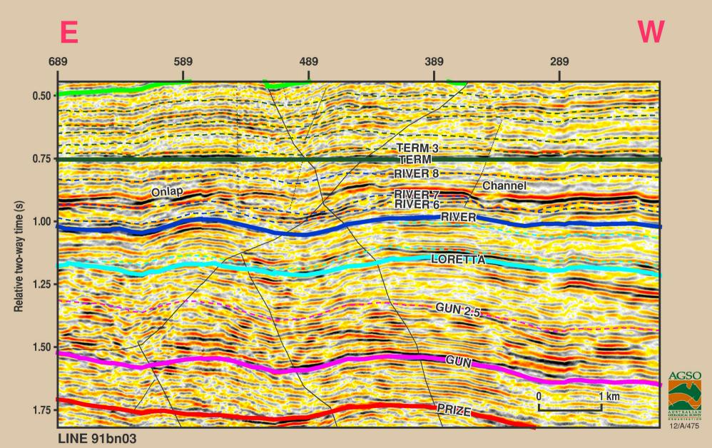
Figure 2.6.4 Seismic sequence stratigraphy of the River supersequence showing channel fill geometry, composite of Line 91bn-03 and 91bn-08 (flattened on Term)
