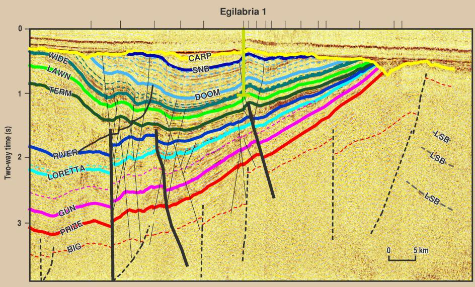
Figure 2.1.5 Egilabria composite section showing geometry of Isa Superbasin phases
