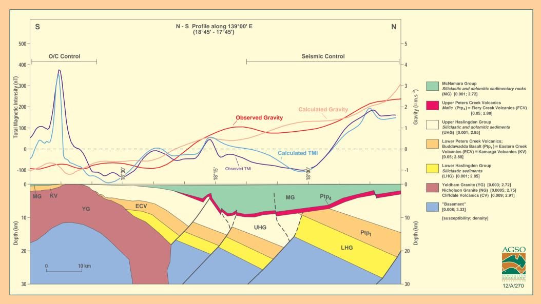
Figure 3.2.4 Geological model from the eastern side of the Comalco seismic grid compared to observed geophysical data
