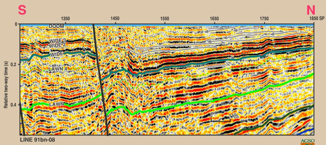
Figure 2.9.4 Seismic sequence stratigraphy of the Wide Supersequence showing onlapping geometry and syndepositional growth, Line 91bn-08 (flattened on Doom)
