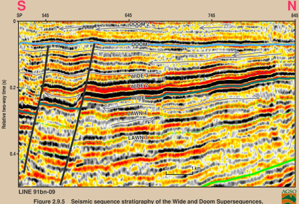
Seismic sequence stratigraphy of the Wide and Doom Supersequences, Line 91bn-09 (flattened on Doom 2) Figure 2.9.5
