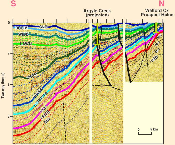
Figure 2.1.2 Argyle Creek composite section showing geometry of Isa Superbasin basin phases
