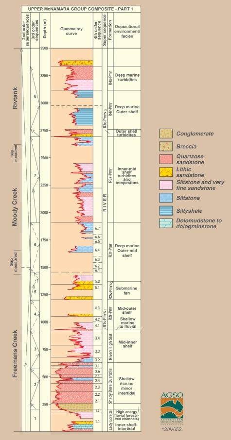
Figure 1.4.2 Composite gamma-ray and lithofacies logs for the River Supersequence
