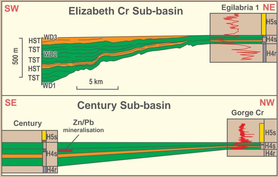
Figure 6.3.3 Comparisons between the geometry and depositional systems in the Elizabeth Creek and Century sub-basins
