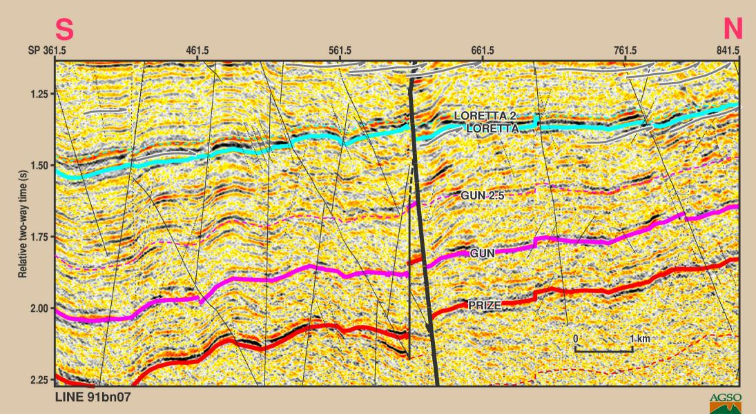
Figure 2.5.1 Seismic sequence stratigraphy of the Loretta Supersequence, Line 91bn-07 (flattened on River). This section is part of the Desert Creek composite (Fig. 2.1.3)
