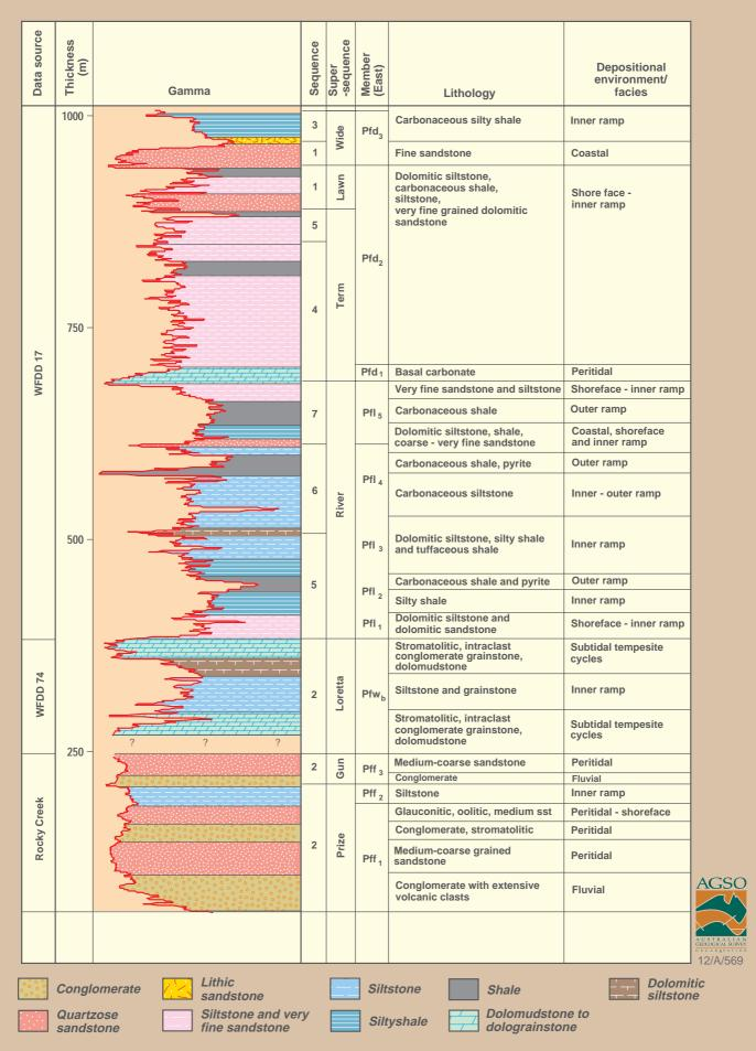
Figure 1.6.1 Sequence stratigraphy of the Fickling Group, eastern Murphy Inlier, based on analysis of composite gamma curve and lithofacies trends
