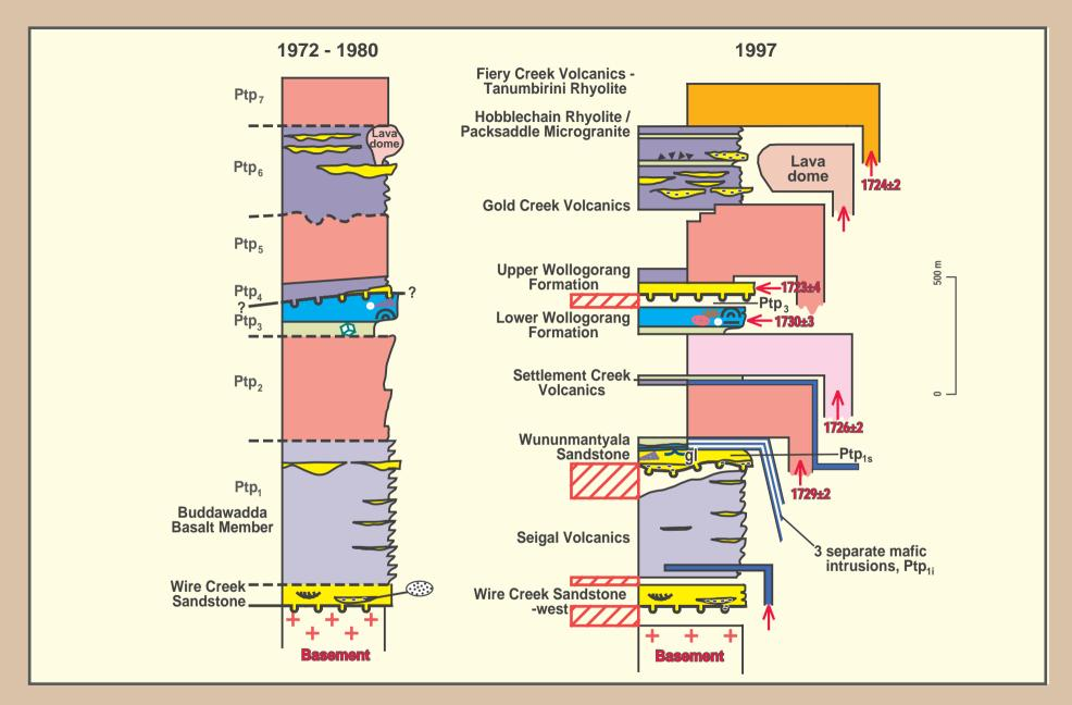
Figure 1.5.2 Stratigraphic columns elucidating the changes to the traditional understanding of the Peters Creek Volcanics on the left resulting from integration of recent regional U-Pb SHRIMP geochronology, palaeomagnetic and field investigations focussed on the Murphy Inlier with existing geochemical and geological data
