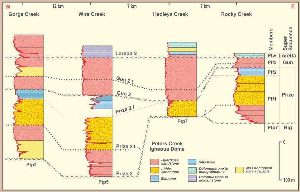
Figure 1.6.3 Cross-section of outcrop logs of the Prize and Gun Supersequences (Fish River Formation) along the Murphy Inlier
