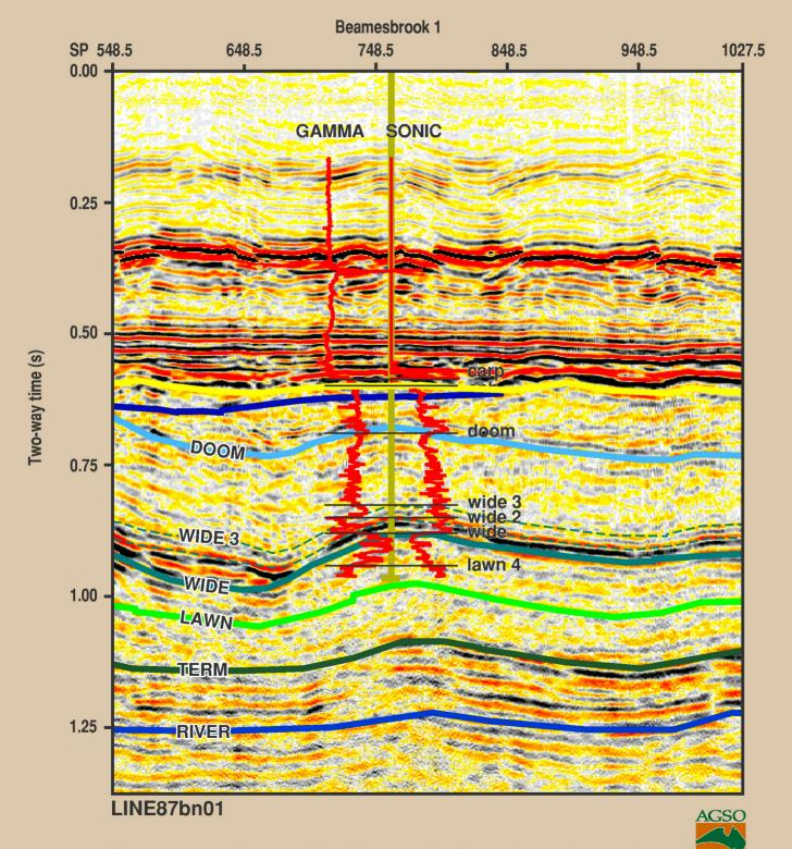
Figure 5.1.5 Beamesbrook 1 well tied to seismic line 87bn-01
