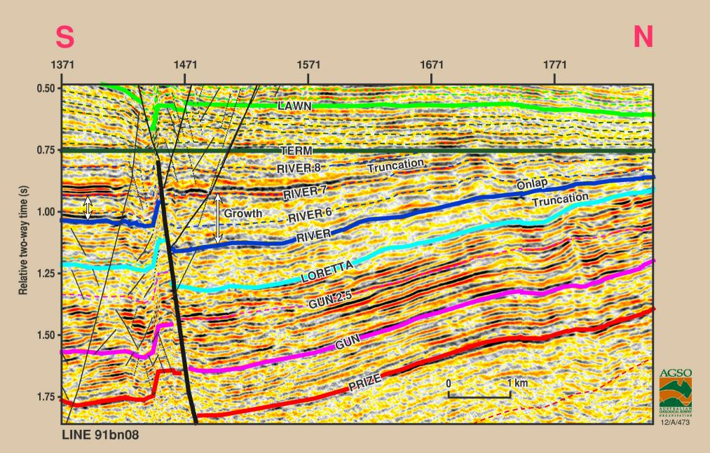
Figure 2.6.1 Seismic sequence stratigraphy of the River and Term Supersequences, showing distinct growth of the River Supersequence across a fault, Line 91bn-08 (flattened on Term)
