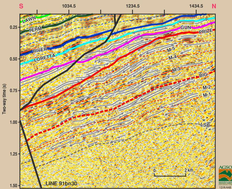
Figure 2.2.1 Seismic sequence stratigraphy of Big, Prize and Gun Supersequences over the Peters Creek magmatic dome line 91bn-30 (unflattened). LSB = Leichhardt Superbasin. M1-M5 relate to magmatic members of the Peters Creek Volcanics. This section comprises the northern end of the Argyle Creek composite Line (fig. 2.1.2)
