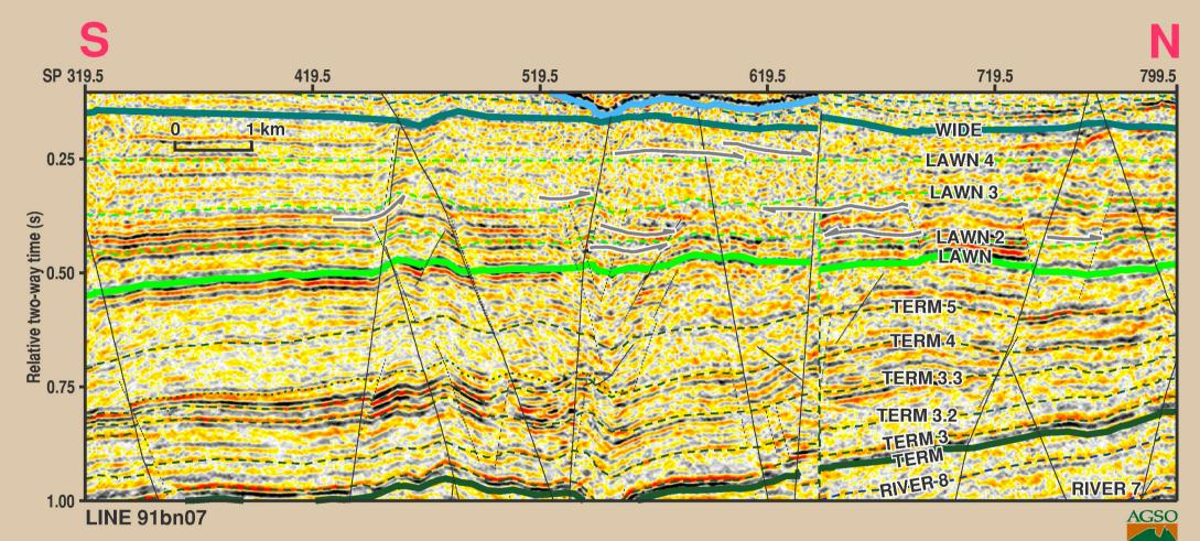
Figure 2.8.2 Seismic sequence stratigraphy of the Lawn Supersequence, Line 91bn-07 (flattened on Lawn 4)
