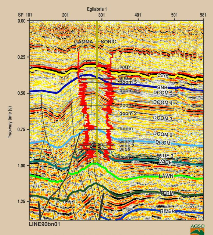
Figure 5.1.4 Egilabria 1 well tied to seismic line 90bn-01
