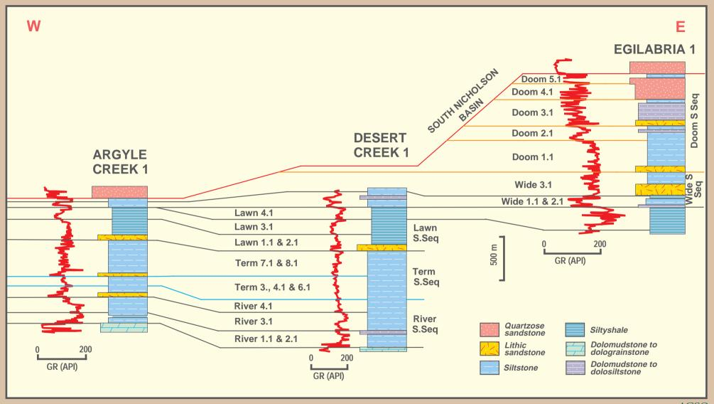
Figure 1.7.3 Evidence for extensive erosion of Isa Superbasin beneath the South Nicholson Group in Comalco well log data
