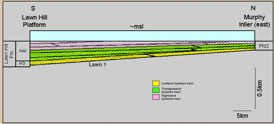
Figure 5.5.6 Sequence stratigraphic model for deposition of Lawn 1 sequences
