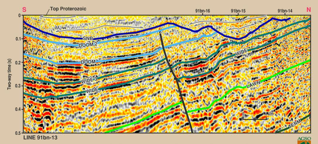
Figure 1.7.2 Seismic geometry of South Nicholson Basin (SNB) overlying the Isa Superbasin in northwestern Lawn Hill Platform. The base of the South Nicholson Group is erosional, and most of the Doom Supersequence has been removed
