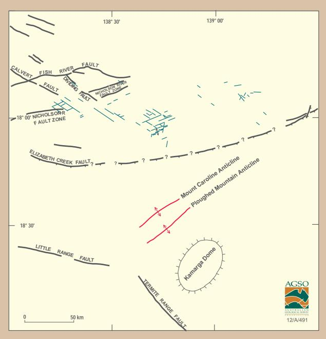
Figure 3.1.1 Late Stage Structures in the northern Lawn Hill Platform
