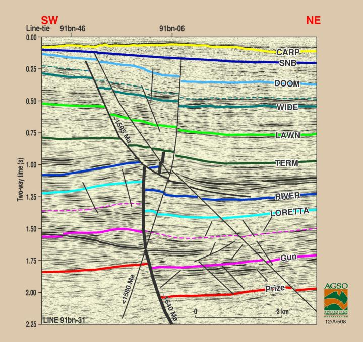
Figure 3.5.2 Interpreted three stage fault system
