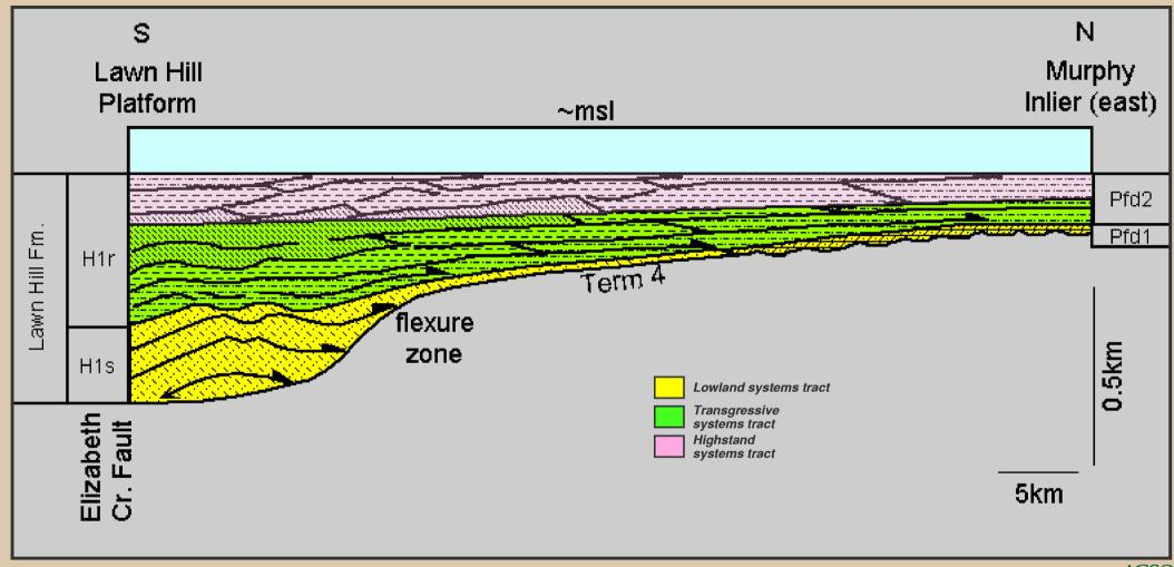
Figure 5.5.4 Sequence stratigraphic model for deposition of Term 4 sequences
