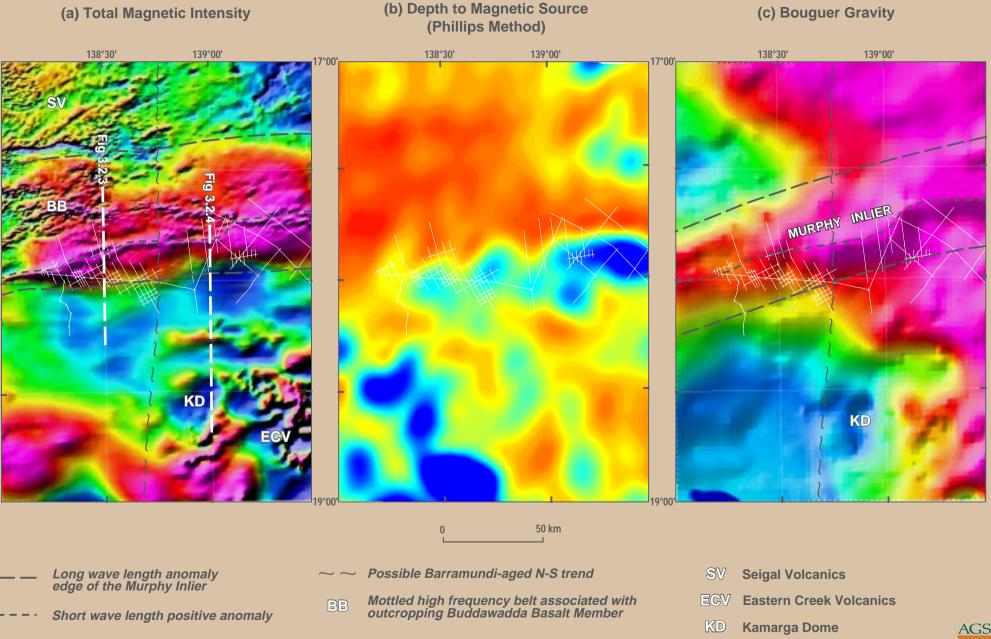
Figure 1.5.1 Geophysical images of the Westmoreland and Lawn Hill 1:250,000 map sheet area (a) Total Magnetic Intensity Image (b) Depth to magnetic sources using the Phillips Deconvolution Method (c) Bouguer Gravity Image
