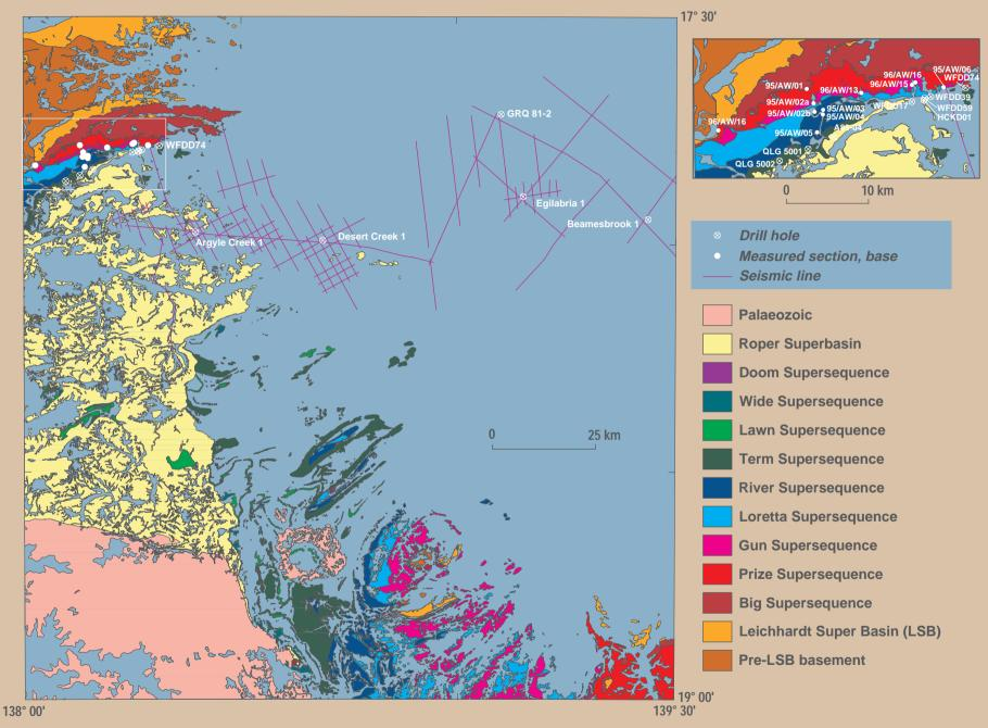
Figure 1.1.1 Geology map with formations grouped at supersequence level with seismic line, well and outcrop section locations shown. Inset shows detail of outcrop sections
