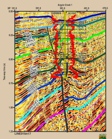
Figure 5.1.2 Argyle Creek 1 well tied to seismic line 91bn-17
