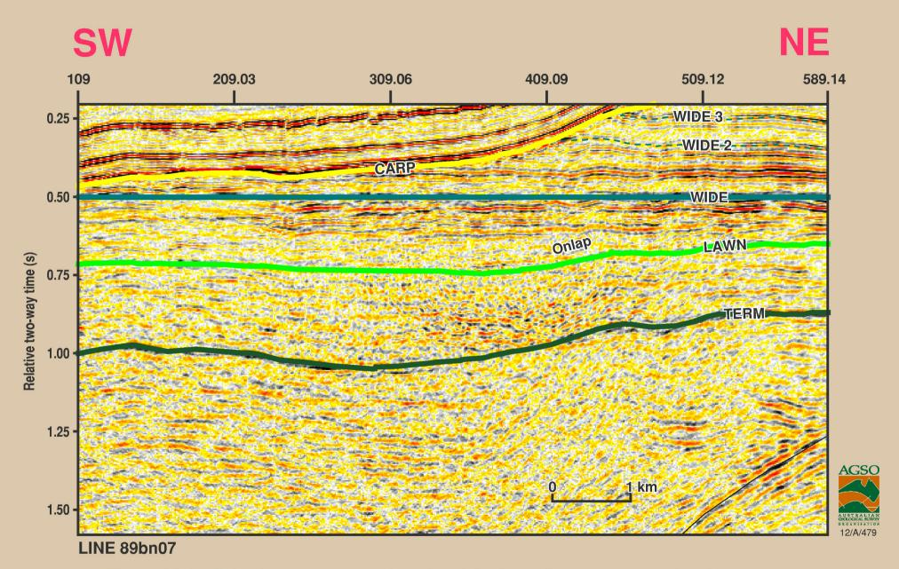
Figure 2.8.1 Seismic sequence stratigraphy of the Lawn Supersequence showing onlapping geometry, Line 89bn-07 (flattened on Wide)
