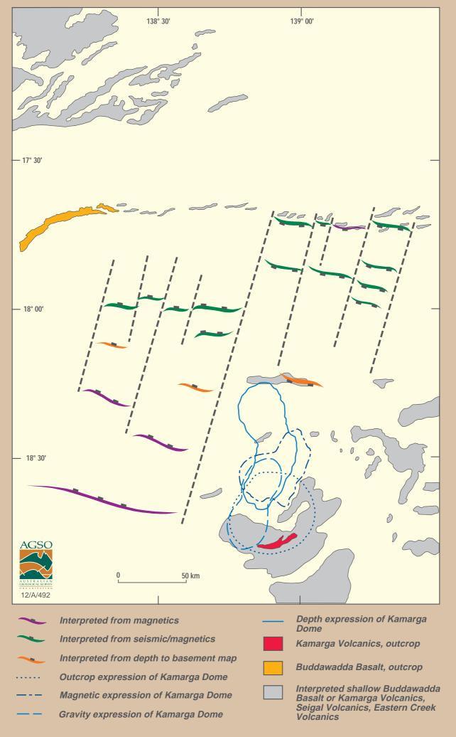
Figure 3.2.1 Basement structures in the northern Lawn Hill Platform
