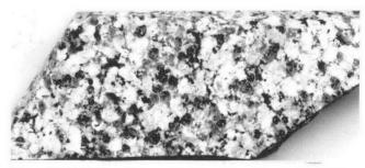
Figure 9.10. Pink, medium-grained, equigranular granite of the Bindogandri Granite. (GR 626890 mE 6335150 mN) Length of sample approximately 60 mm. (O.L. Raymond photograph)
