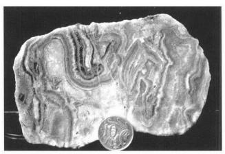
Figure 6.3. Crustiform-colloform banded quartz boulder from the base of the Manna Conglomerate, overlying Girilambone Group rocks north of Condobolin. (GR 511650 mE 6345800 mN) (O.L. Raymond photograph)
