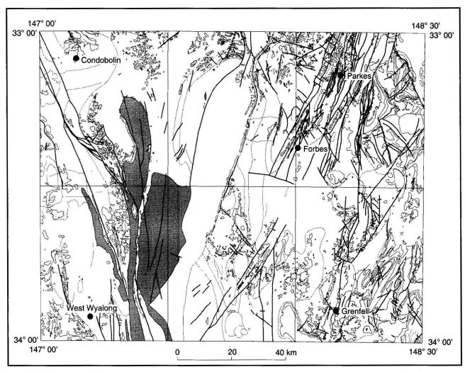
Figure 3.15. Distribution of the Lake Cowal Volcanic Complex in the Forbes 1:250 000 map sheet area. Areas shaded black represent substantial outcrop. Areas shaded grey represent distribution beneath surficial cover.
