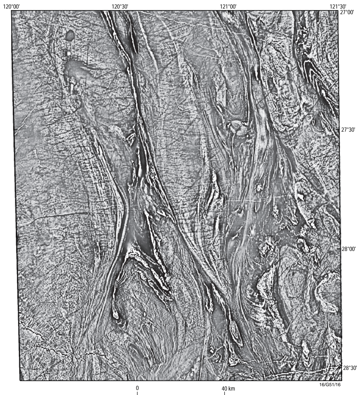
Figure 4. Greyscale first vertical derivative of total magnetic intensity image of the Sir SAMUEL and northern part of the LEONORA 1:250 000 sheet areas
