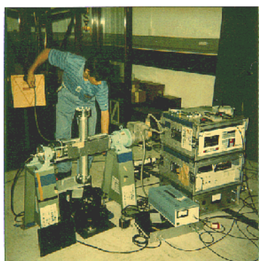
Absolute gravity measurements March 1993 by National Astronomical Observatory Mizusawa Japan.
