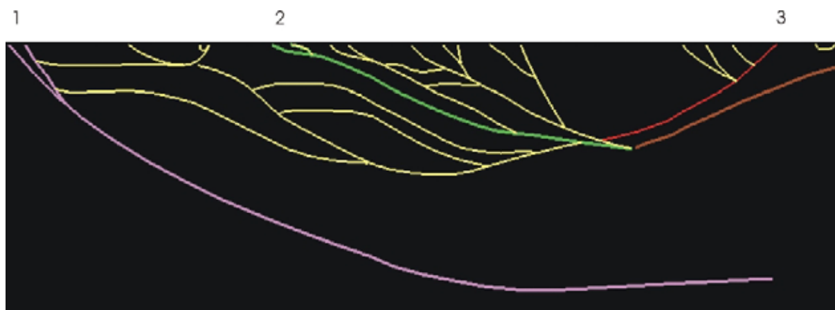
Figure 5 Example of the final iteration of the cross sections (same area as Figs. 3, 4), following input of seismic reflection geometry. Note the shallow dips, and relatively shallow greenstone. 1 - Mt George shear zone, 2 - Kilkenny shear zone, 3 - Murrin fault
