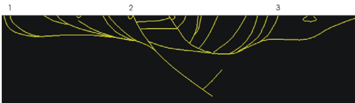
Figure 4 Example of the second iteration of the cross sections (same area as Fig. 3). Note the generally steep dips, and shallowing of the greenstone. 1 - Mt George shear zone, 2 - Kilkenny shear zone, 3 - Murrin fault
