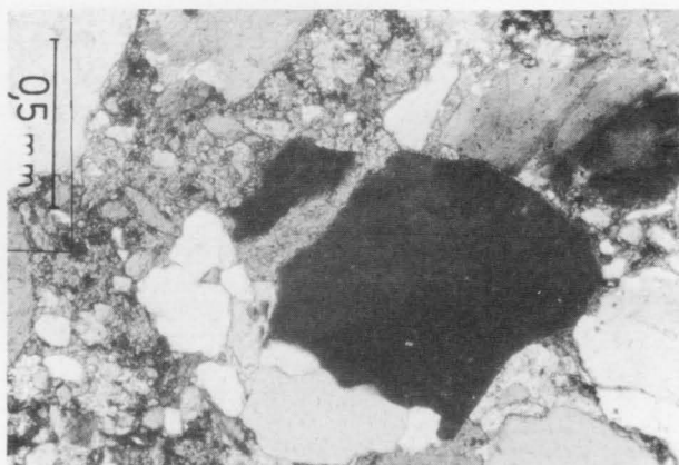
Figure 12f. Calcite replacing quartz in a quartzite fragment; Yellow Drum Sandstone, BMR Lennard River 1 (locn WCB LR1/107) x 58
