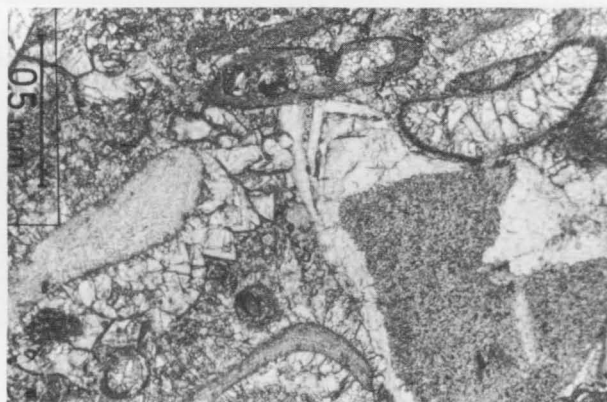
Figure 16f. Syntaxial cement rim extending from crinoid ossicle on a skeletal grainstone; Laurel Formation, type section (locn WCB 102/1) x 58
