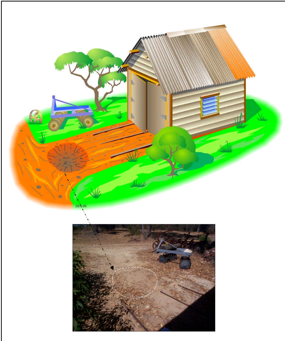
Figure 3.2 Photo and schematic picture of the hole on the Trian St property. The white circle marks a slight depression where the hole formed.
