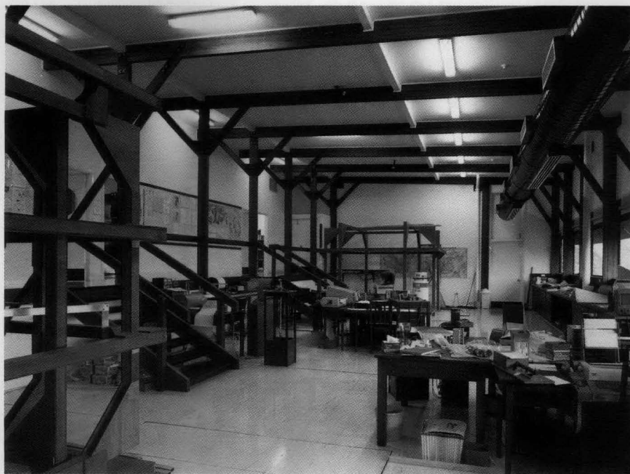
Figure 3. CSIRO North Ryde (Sydney) laboratory, showing Helmholtz coil sets for the cryogenic magnetometer (background) and the furnace (foreground).
