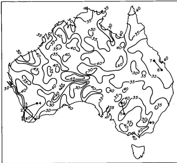
Figure 8. Predicted crustal thickness for Australia assuming 1^\circ \times 1^\circ areas are in complete isostatic equilibrium. Contour interval 5 km. The numbered refer to seismic traverses of Fig. 9.
