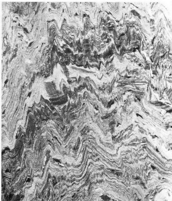
Figure 9. Carbonaceous (dark grey) mica-quartz schist with pervasive S_2 crenulation cleavage and large phlogopite porphyroblasts. Cahill Formation lower member. Plane-polarized light x 5.
