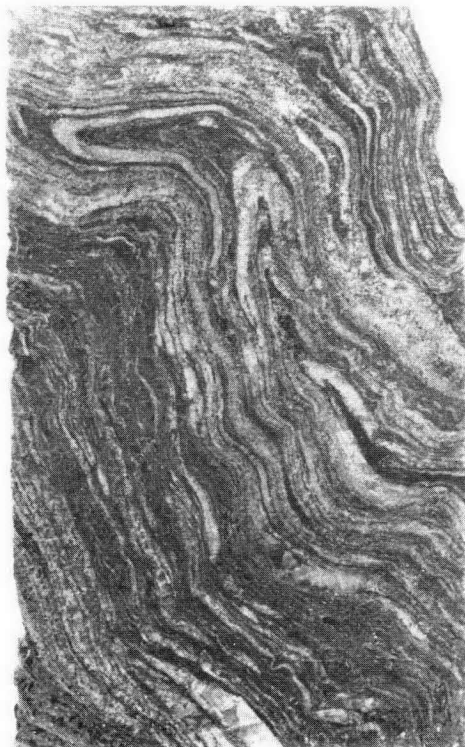
Figure 15. Strongly deformed mica-quartz schist of Fisher Creek Siltstone shows a complex deformational history: compositional layering ( S^0 ) is isoclinally folded and virtually parallel to the axial plane ( S^2 ), which is openly folded by crenulation cleavage S^3 . Black flecks in extreme bottom left are magnetite. x 1.
