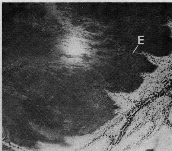
Figure 2. Clear 'dumped' stormwater (shown by sun reflection) on the grassed plain, and silty 'imported' floodwater in the drainage system.
