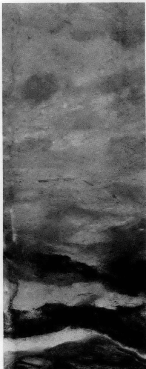
Figure 8. Radiograph (positive, natural scale) of core 35 KL (Facies 4).
