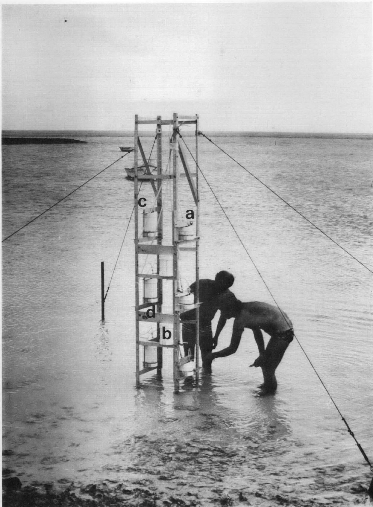
Figure 1. Tower system used to collect suspended sediment samples at One Tree Reef. (a) rising tide sample containers; (b) PVC float containers for release mechanism; (c) falling tide sample containers; (d) housing for release mechanism.
