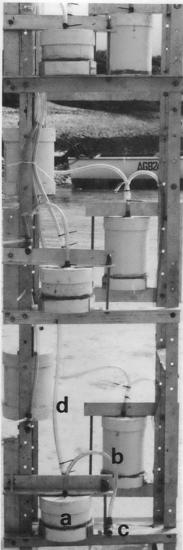
Figure 3. Operation of falling tide sampling mechanism. A. operating lever locked in position by rotating aluminium block; B. rotating block released—tubing remains closed; C. rubber tubing opened and air expelled.
