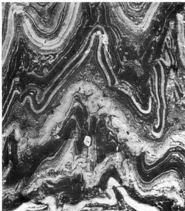
Figure 4. Oxidised and partially leached lead-zinc-silver ore from Black Star open-cut, Mount Isa.
