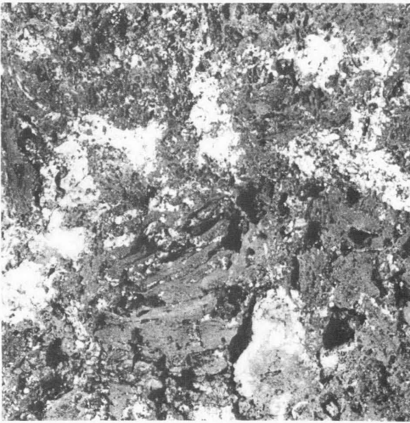
(b) Dark massive gossan with lighter patches of secondary lead minerals of alunite-jarosite series (3 cm across).
