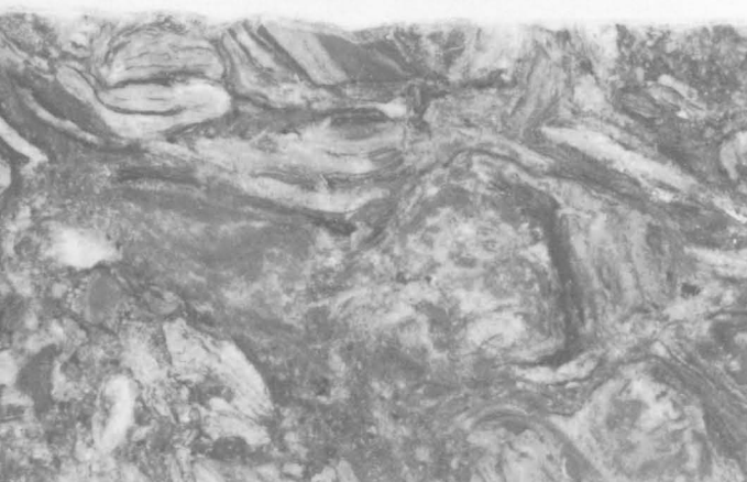
Fig. 30. Slabbed section of core showing contorted laminae of gypsiferous dolomite (black) and fragments of light brown tough dolomite (grey) in brecciated and contorted gypsum; from 38.31 m. x 1. (GA/4319)
