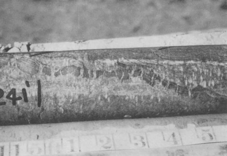
Fig. 31. Steeply dipping lamina of light brown tough dolomite (grey) in gypsum, showing boudinage structure. Fractures are filled with acicular gypsum from 73.51 m. x 1. (GA/4787)
