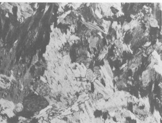
Fig. 28. Gypsum (light grey to black) showing felted texture and sparse dolomite crystals (grey rounded); from 33.91 m. Crossed nicols, x 60. (M/1195-36)
