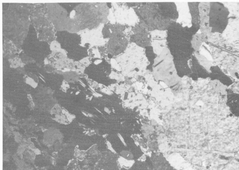
Fig. 20. Medium to coarse-grained anhydrite, showing lamellar twinning and cleavage traces. Quartz euhedra also visible; from 169.62 m. Crossed nicols, x 41. (M/1289)
