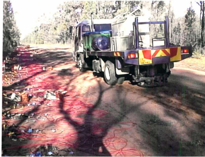
Figure 3. T15000 Minivib vibrating next to the receiver line.
