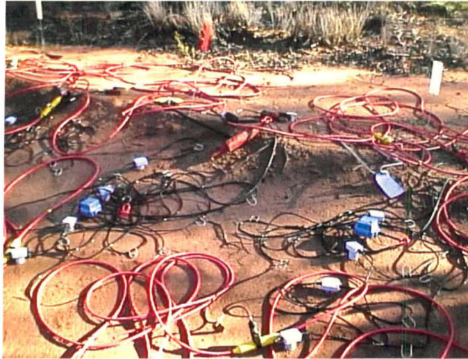
Figure 4. 10 Hz geophones strings (groups of 4) and the larger 3-component geophones.
