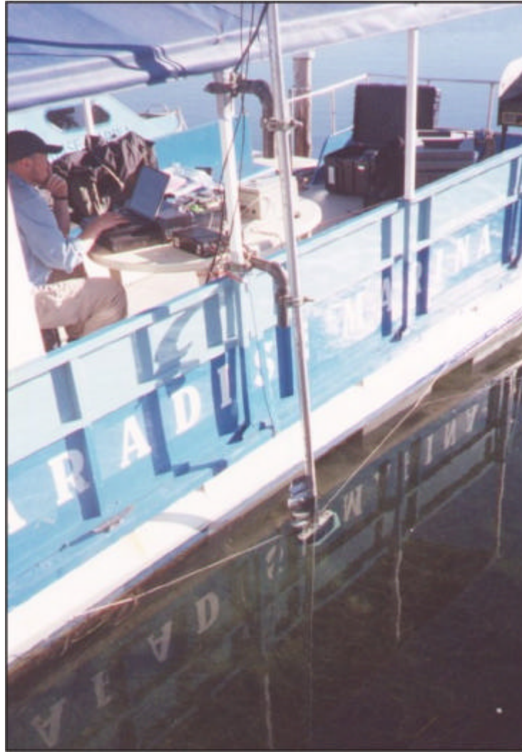
Figure 4 - Installation of the QTC system. The transducer and DGPS antenna were installed on an aluminium pole mounted upon the side of the boat.
