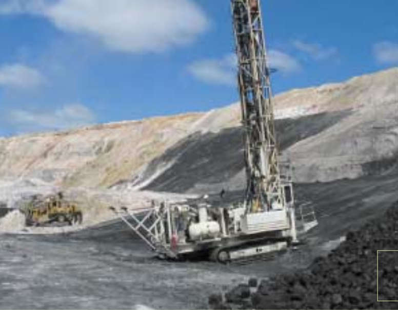
Griffin Coal's Muja mine near Collie (WA). Bulldozer cleaning-off seam prior to drilling and blasting (Geoscience Australia, Bill McKay).
