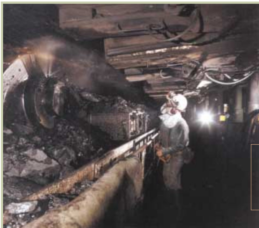
Longwall mining operation at the Newstan Colliery near Newcastle, New South Wales (Centennial Coal Co Ltd)
