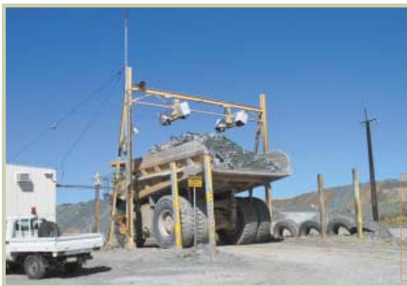
Radiometric discriminators used to measure the average uranium grade of ore in haul truck, Ranger mine, Northern Territory (Geoscience Australia, Aden McKay)
