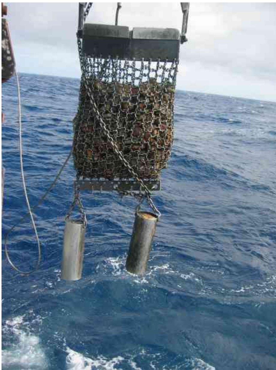
Figure 3.4 A photograph showing the dredge equipment being recovered after a successful deployment during Survey 265 on the Southern Surveyor.
