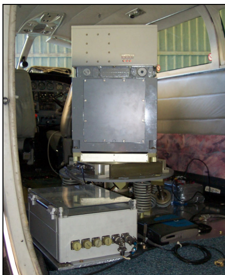
Figure 1. Photograph of the GT-1A gravimeter installed in a Cessna 404. The gravimeter sits on a brass-coloured rotating table, which in turn sits on the shock mount. In the left foreground is the uninterruptible power supply (UPS), and to its right is a small blue Z-Surveyor dual frequency GPS receiver.
