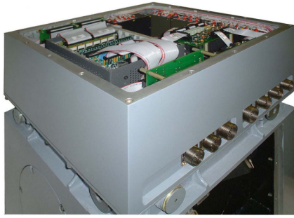
Figure 2. Photograph of the GT-1A gravimeter from above, with cover removed showing the electronics bay.
