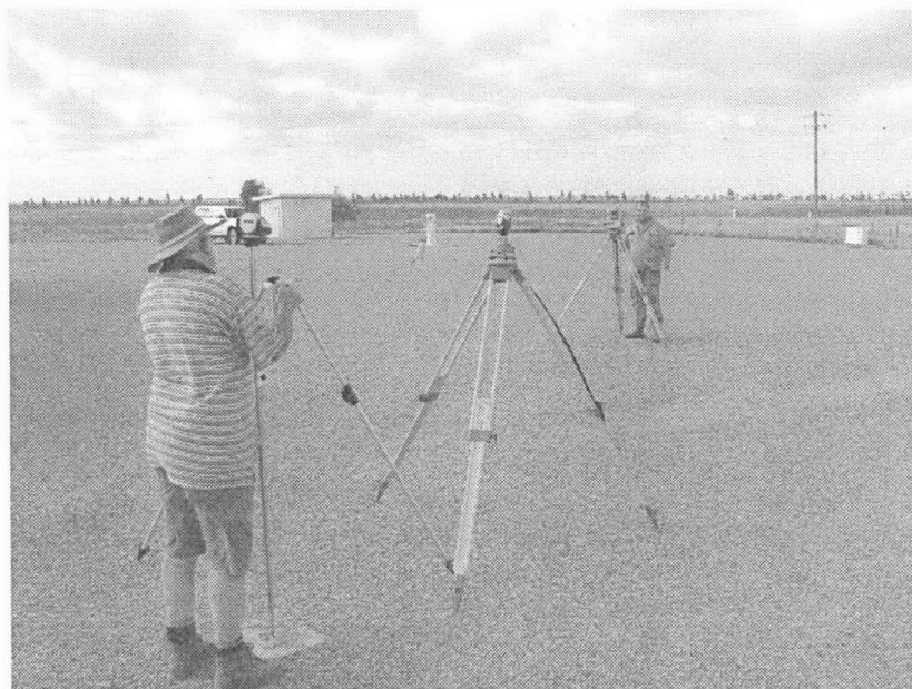
Figure 11: Yarragadee levelling; fixed height prism pole braced by a bi-pole used for EDM-height traversing technique.
