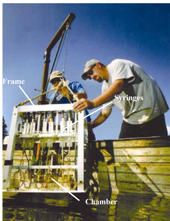
Figure 2-3. Deploying an automatically sampled chamber. Spring-loaded syringes are arranged around the chamber and supported by the frame. (Photo: Newcastle Herald).
