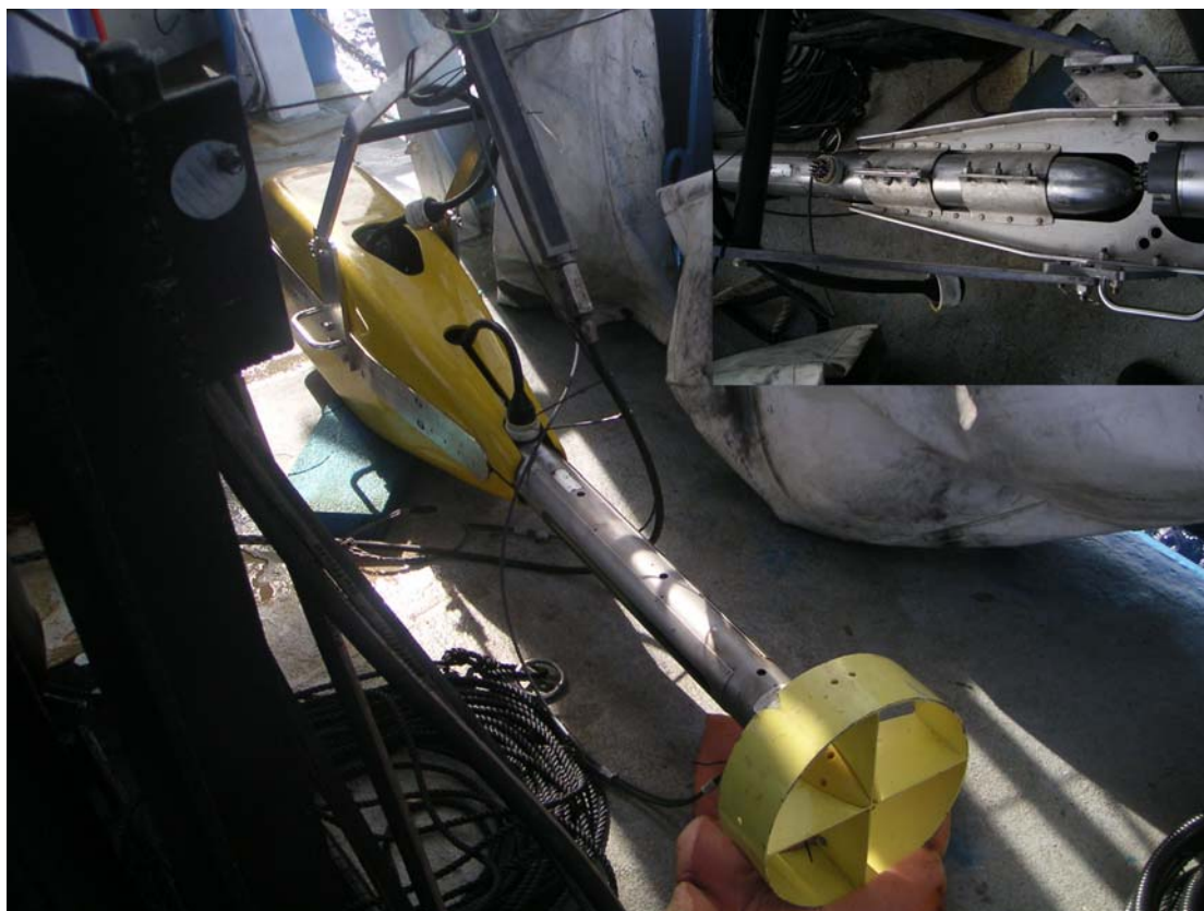
Figure 2.3. The sidescan/sub-bottom profiler used on the survey. Inset shows the sidescan fish (metal cylinder) mounted inside the profiler head
