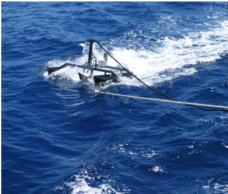
Figure 2.4. Skimmer device constructed by GA technical staff to sample the sea surface and supply sampled water to the fluorometer.
