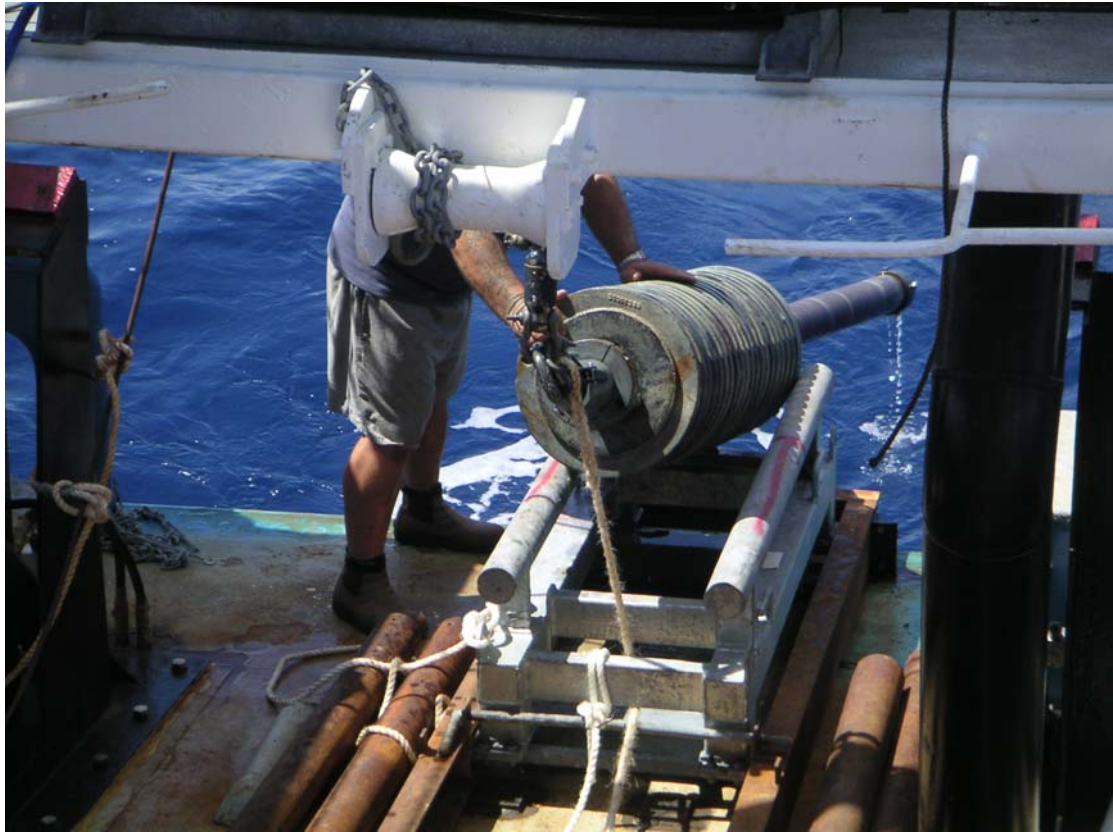
Figure 2.9. Deploying the gravity corer. Note the slightly bent bomb
