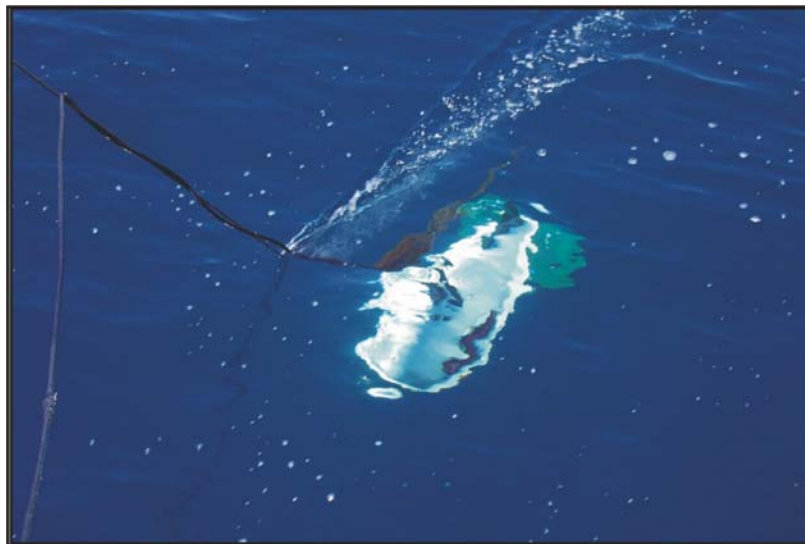
Figure 2.4. Photograph of the Chirp (3.5kHz) seismic reflection tow-fish. The tow-fish was towed behind the vessel approximately 3 m below the water surface at 9-11 km hr -1 in smooth to slight seas.
