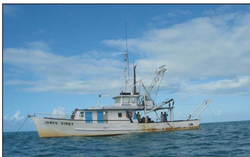
Figure 1.4. Photograph of the RV James Kirby . The vessel is a 20 m long converted fishing trawler owned and managed by James Cook University in Townsville.
