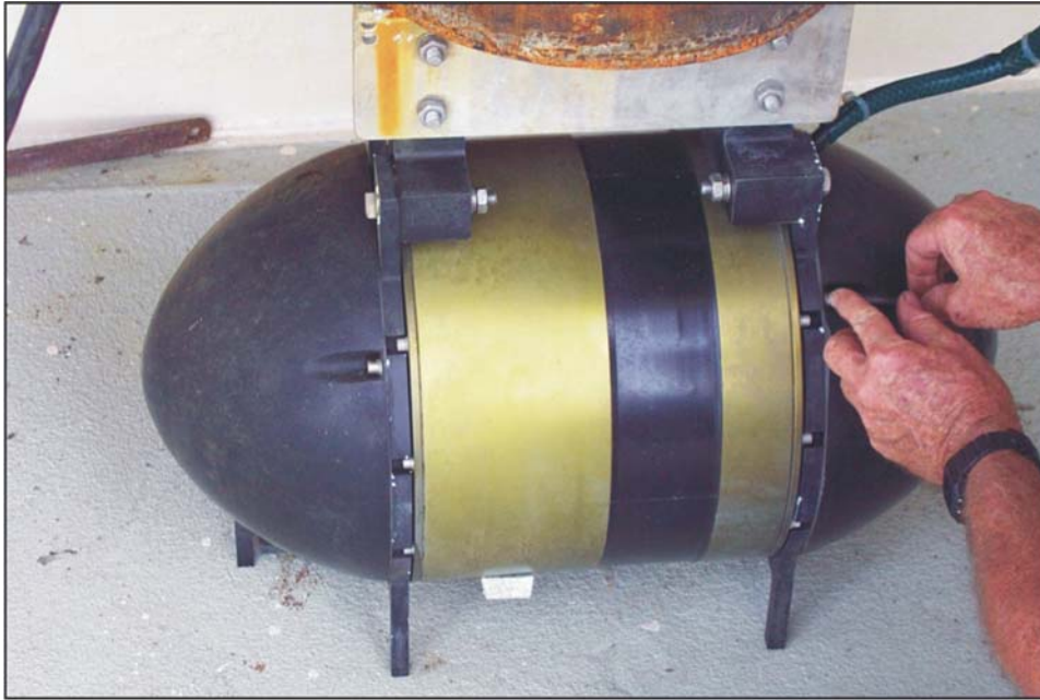
Figure 2.2. Photograph of the Reson 8101(240 kHz)multi-beam sonar transducer/receiver. The unit is attached to a vertical pole on the starboard side and projects approximately 1.5 m below the hull of the vessel. The unit emits and receives 101 beams to obtain bathymetry and acoustic backscatter.
