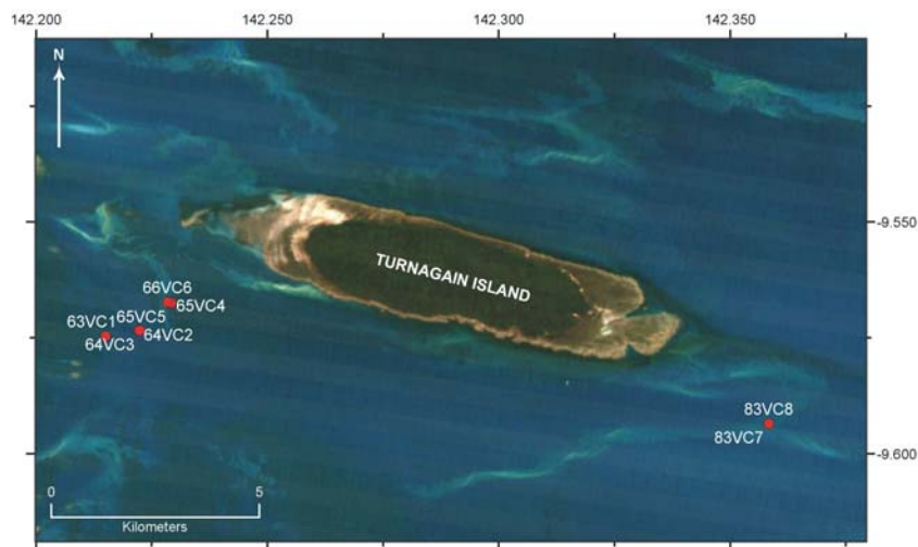
Figure 4.12. Map showing the location of the vibrocores. The vibrocores were located on the crests of the sand ridges in Area A and prominent sandwaves in Area B to sample any internal bedding surfaces that could depict historical changes in the orientation of the dunes, and to provide samples for analysis of physical properties of the sediment. No internal structures or changes in texture and composition were observed in the cores. Details of the vibrocores recovered during the survey are located in Table 4.3. The core logs are provided in Appendix H and textural and compositional data for the sub-surface samples are reported in Appendix I.
