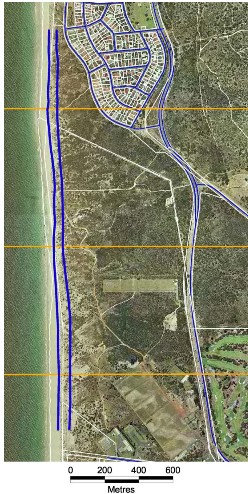
Figure 7.11: Swanbourne Beach, southwestern Western Australia, showing the current position of the coastline and the potential coastline position given the recession calculated with the Bruun Rule
