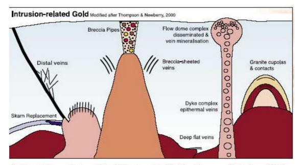
Figure 1. Generalised model for IRG systems. Modified from Thompson & Newberry (2000), to include breccia pipe (Kidston, Qld: Baker & Andrew 1981) and granite carapace (Timbarra, NSW: Mustard 2001) styles.
