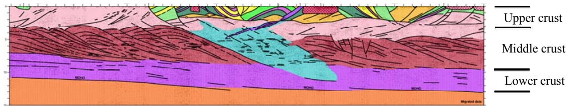
Figure 8-64: 91BMREGF01 seismic line, from Drummond et al. (2000) showing mid crustal imbricates (dark red layer). In 3D these imbricates are domical.
