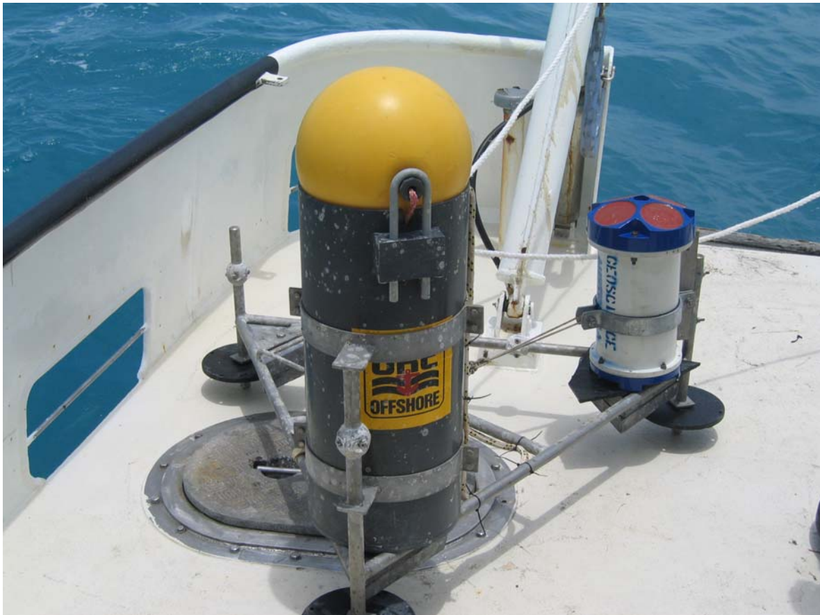
Figure 4.6. Mooring 04CM03 showing acoustic release system (front of image), and ADCP (rear and to the right).
