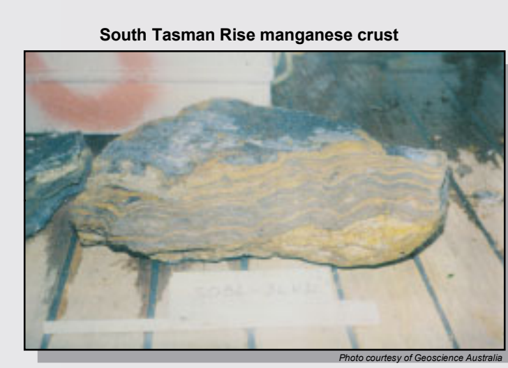
Cross-section through 15 centimetre thick manganese crust from the South Tasman Rise, south of Tasmania. Water depth 3200 metres
