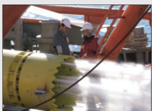
High pressure water jets for seabed sediment (green) ignition during sampling
