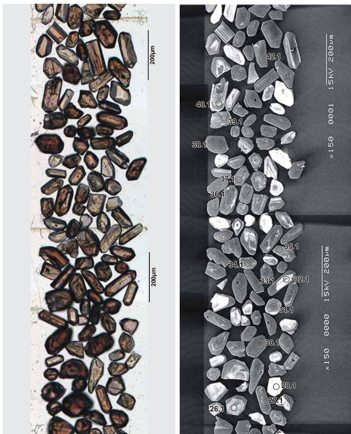
Figure 51. Representative images (transmitted light on left, cathodoluminescence on right) for sample 2004969008: biotite granodiorite, Newlgalup. SHRIMP analysis spots are labelled.
