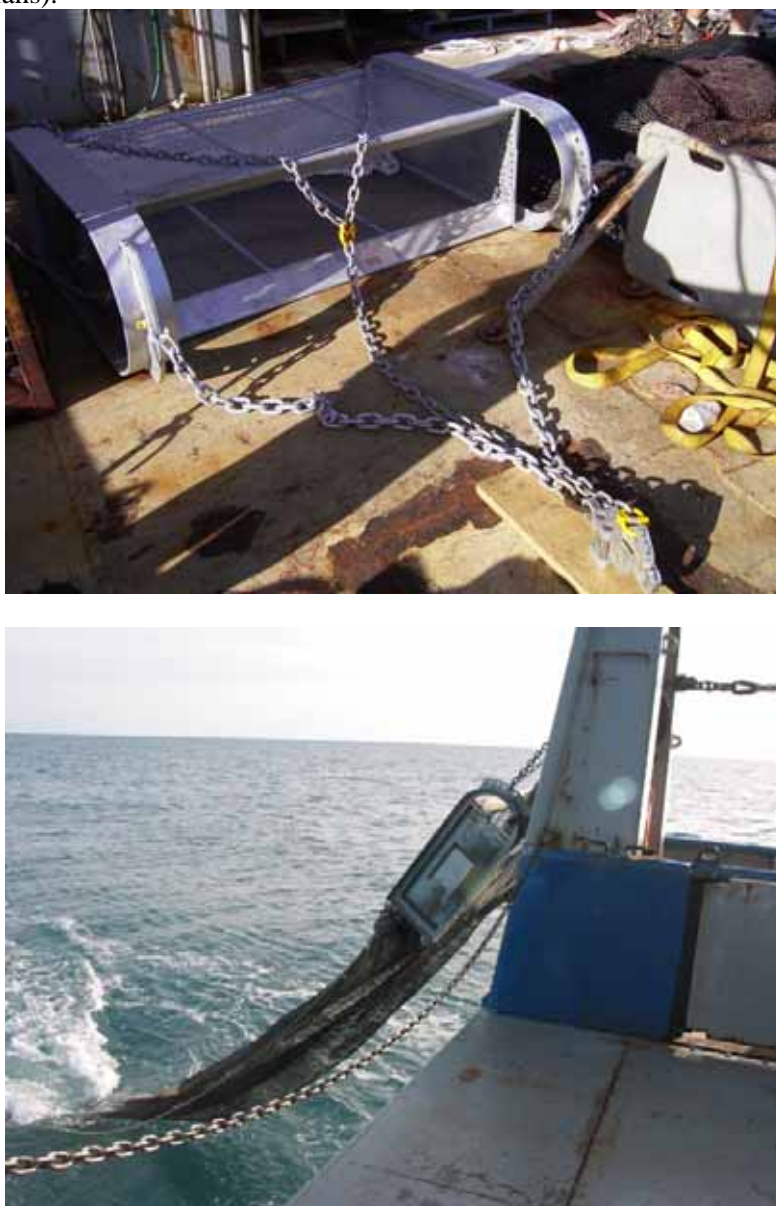
Figure 5.1 Photographs of the benthic sled used for sampling seabed biota.
