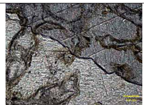
Fig. 4.16 (D) G-000175. Photomicrograph showing detail of G-000174. The two calcite crystals, whose boundary is marked by the dark line running from top left to lower right, show envelopment of both coral and pores (Crossed polarisers; scale bar = 100 \mu\text{m} ).
