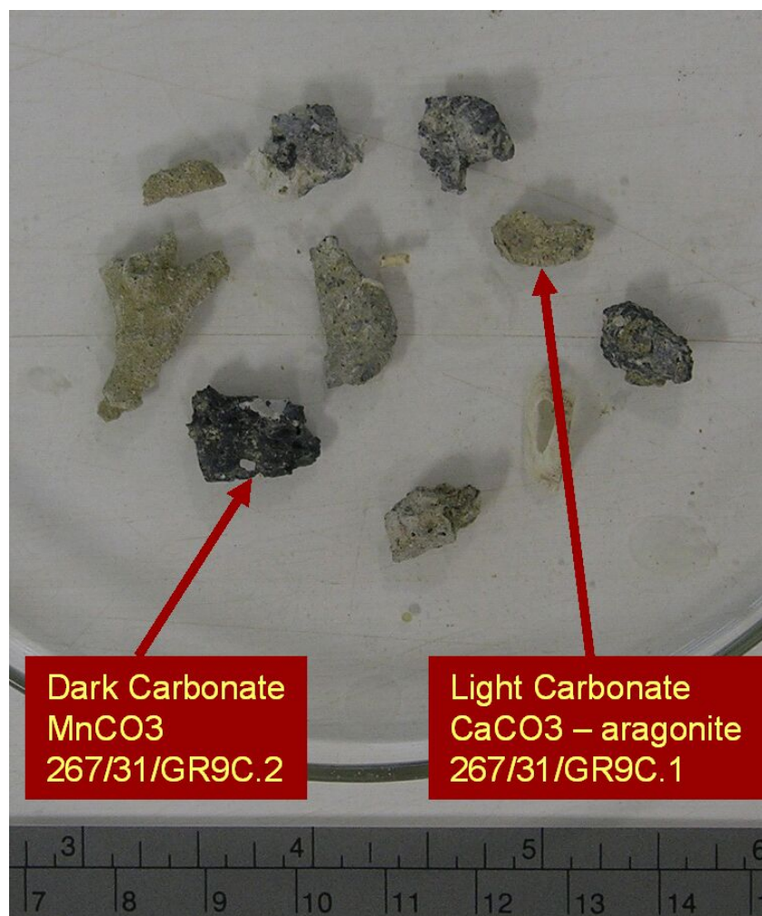
Figure 92. Light coloured carbonate (aragonite) and dark coloured carbonate (MnCO 3 ) was collected from a grab sample (267/31/GR9B).
