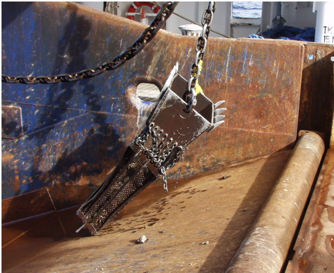
Figure 89. Photo of rock dredge used to sample seabed carbonates and other lithified substrates.
