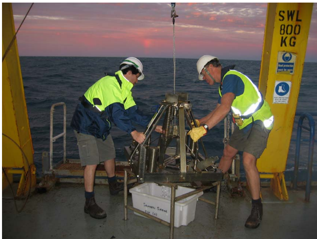
Figure 90. Photo of grab and box cores used to sample seabed sediments.
