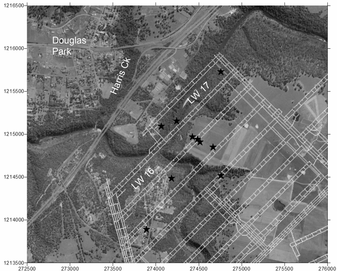
Figure 3. Detail of the Nepean and Cataract Rivers, longwalls 16 and 17 of Tower Colliery, the freeway, bridges and other infrastructure. Harris Creek flows south through a narrow ravine to the Nepean River. It is thought that difficult ground conditions in in-seam drill holes and mine headings in the northwest corner of LW16 are due to a northerly continuation of a north-south trending fault encountered further south in Tower Colliery. Black stars indicate locations of some of the seismic events detected during the period September 1999 to January 2000.
