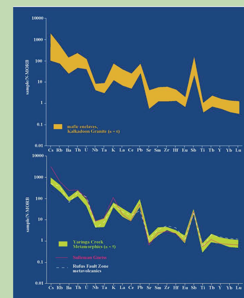
N-MORB-normalised incompatible element plots for pre-1820 Ma basement rocks from east and west of the Mt Isa Fault
