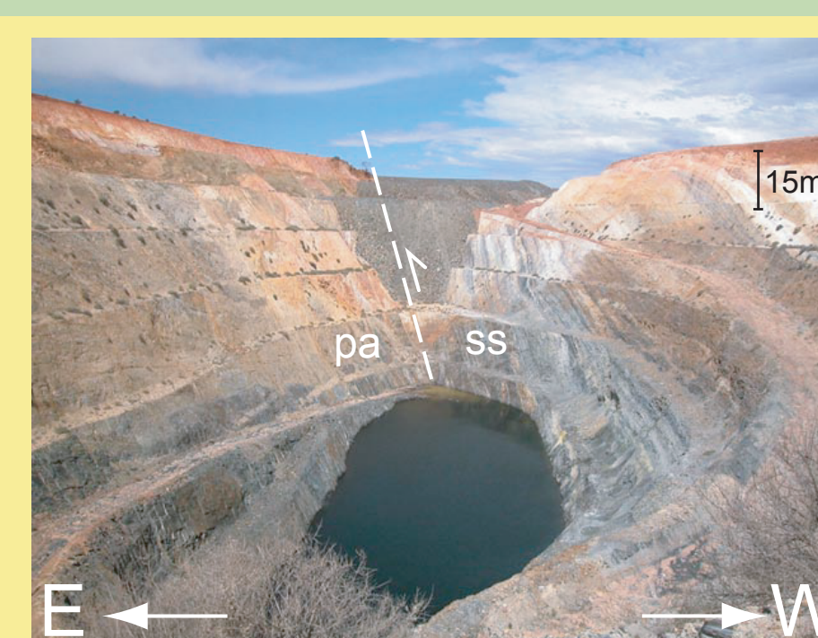
Figure 2(b): Yunnadaga, looking south. Westerly-dipping sandstones and shales (ss) in fault contact with a more competent para-amphibolite unit (pa). Lode-Au structures are observed along this contact.
